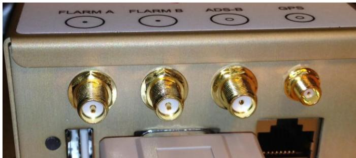
FLARM A and B Ports are reverse polarity female SMA connectors, with a (male) pin as centre conductor. ADS-B is a standard female SMA connector with a female centre receptacle.
