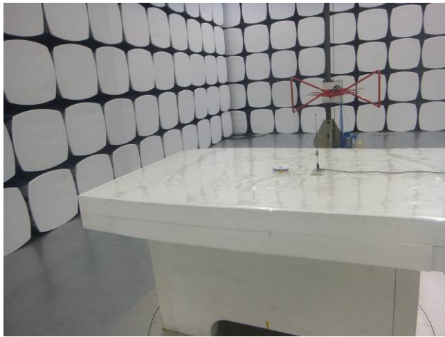
Radiated Spurious Emissions Test Setup Below 1GHz
