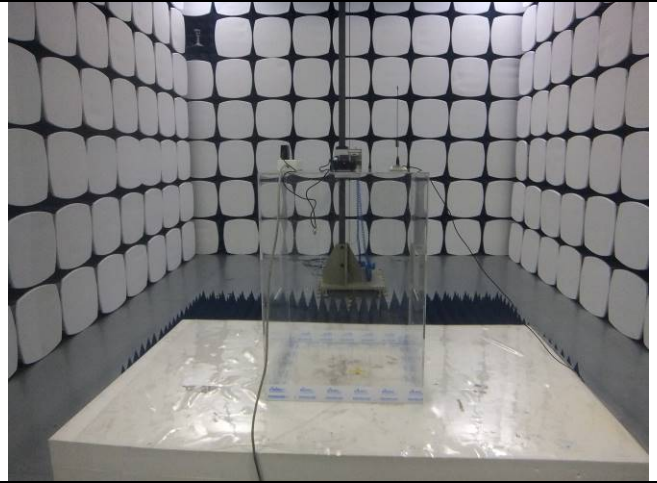
Radiated Spurious Emissions Test Setup Above 1GHz
