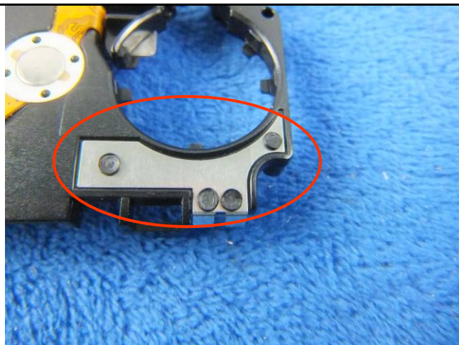
WIFI - Antenna View
