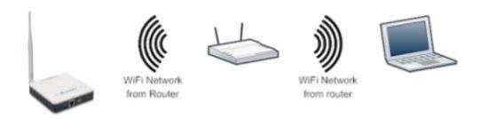
If the LPS8N already connect to the router via WiFi, use can use the WiFi IP to connect to LPS8N.
