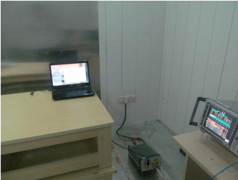
FCC RADIATED EMISSION TEST SETUP
