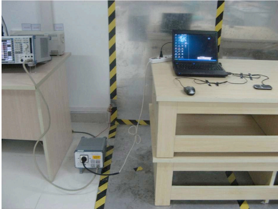
FCC LINE CONDUCTED EMISSION TEST SETUP
