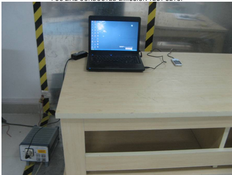
FCC LINE CONDUCTED EMISSION TEST SETUP
