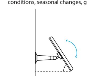
2. Mount the bracket with the mounting template and the screws provided in the package.
