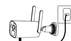
**⚠** Please use a standard included high-quality DC 5V/2A adapter to charge the battery. If using a low-quality adapter may be incompatible or the charging time may be too long.
