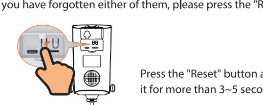
Press the "Reset" button and hold it for more than 3-5 seconds
