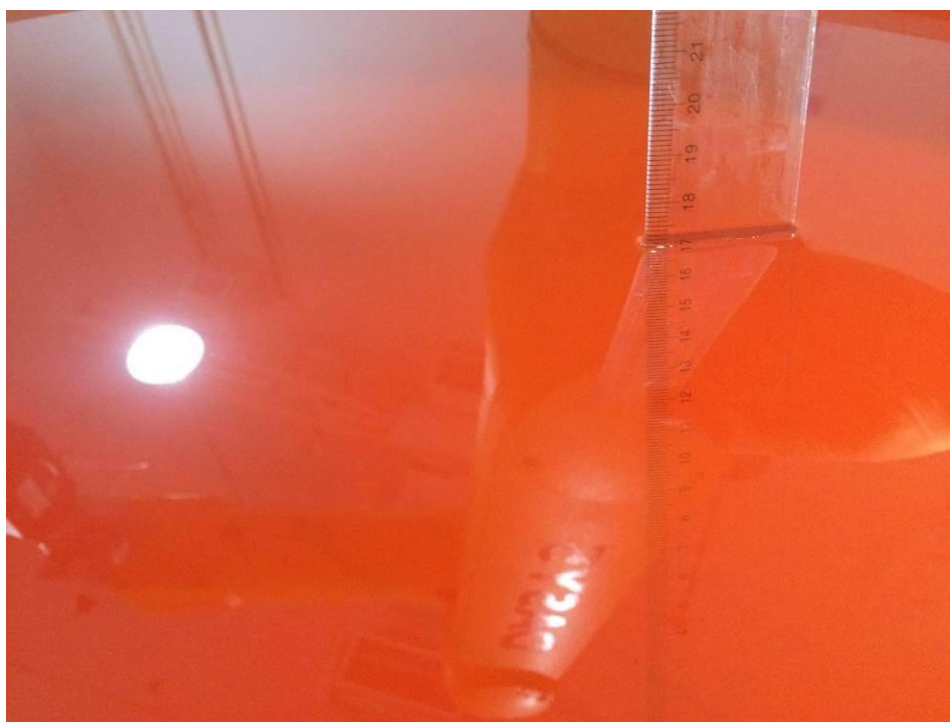
Picture 9-8: Liquid depth in the Flat Phantom (2450 MHz Body)
