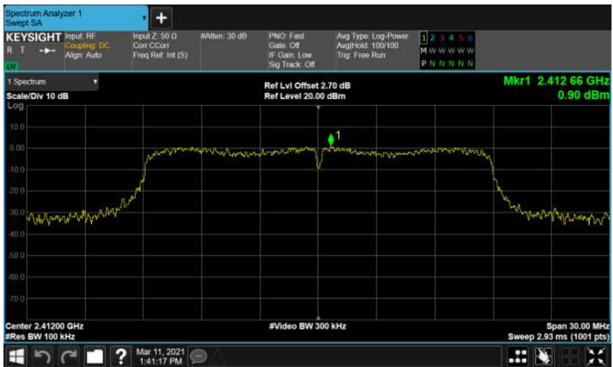
Band Edge NVNT n20 2412MHz Ant1 Emission
