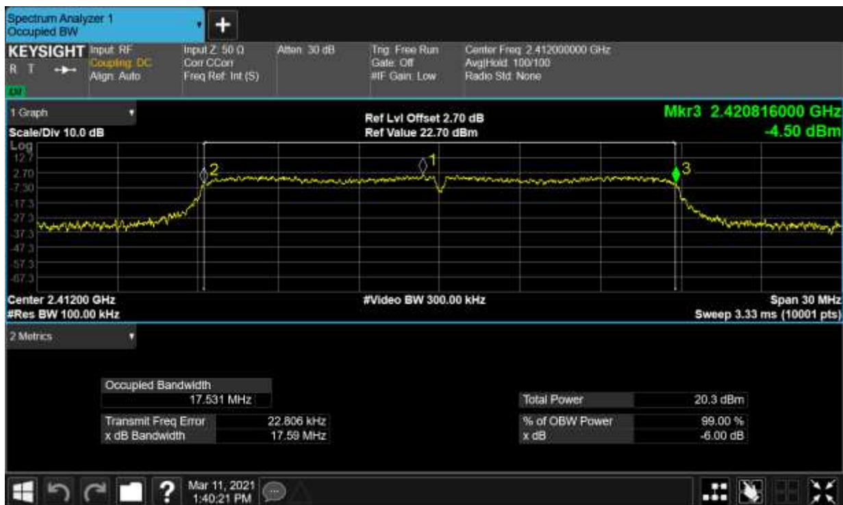
-6dB Bandwidth NVNT n20 2412MHz Ant2
