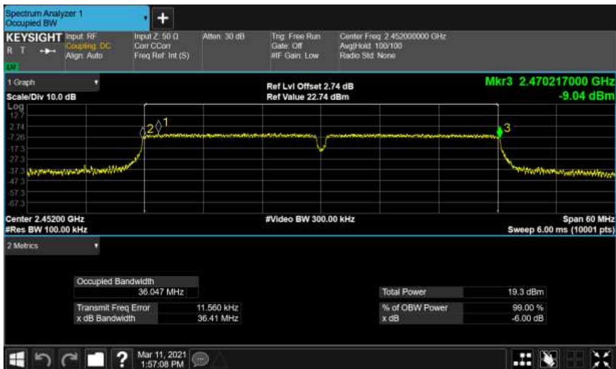
-6dB Bandwidth NVNT n40 2452MHz Ant2
