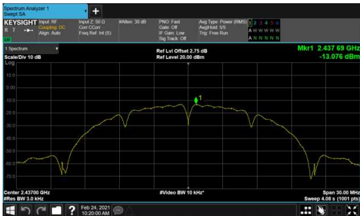
PSD NVNT b 2462MHz Ant2
