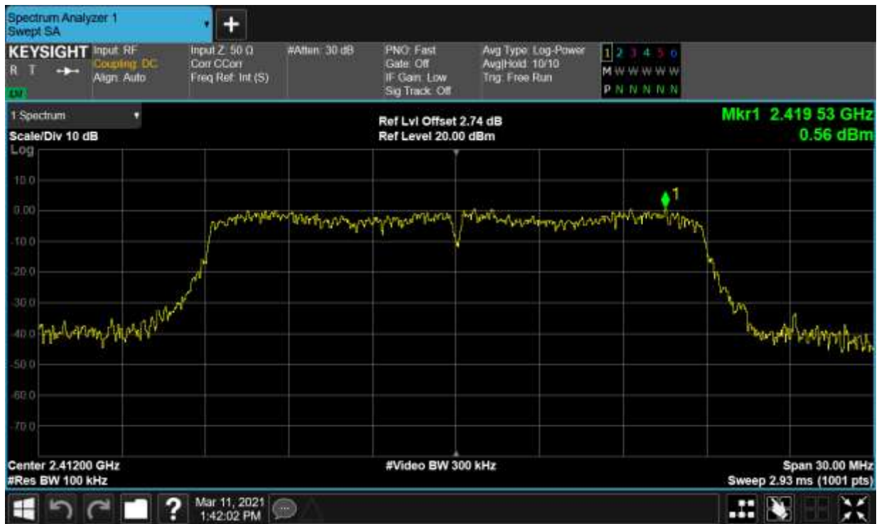
Tx. Spurious NVNT n20 2412MHz Ant2 Emission
