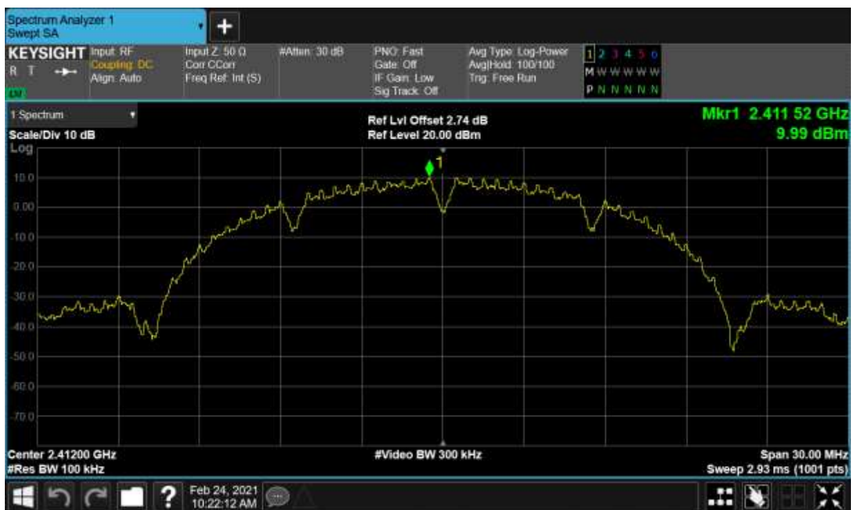
Band Edge NVNT b 2412MHz Ant2 Emission
