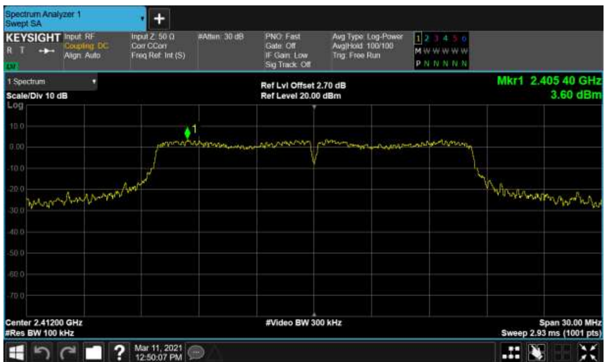
Band Edge NVNT g 2412MHz Ant1 Emission
