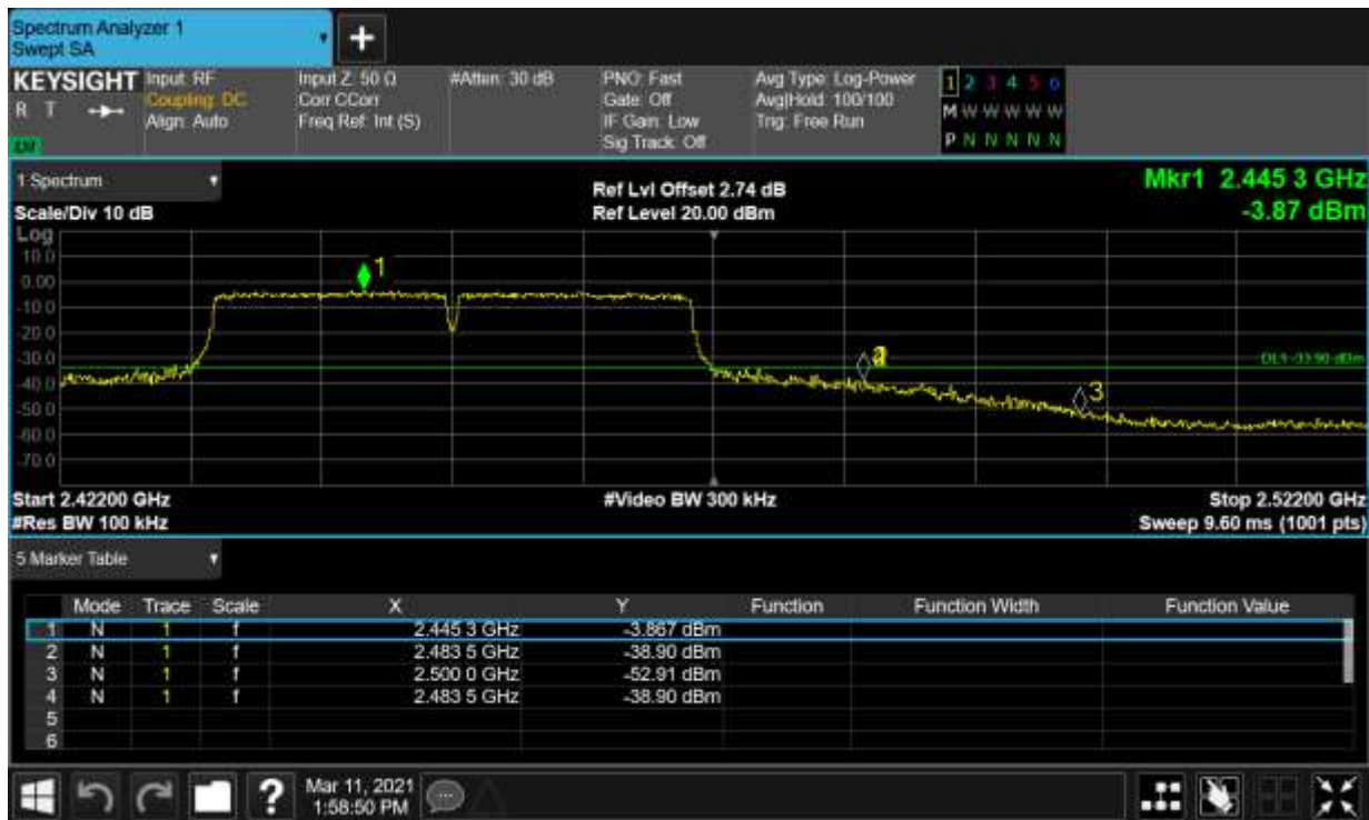
Band Edge NVNT n40 2452MHz Ant2 Ref
