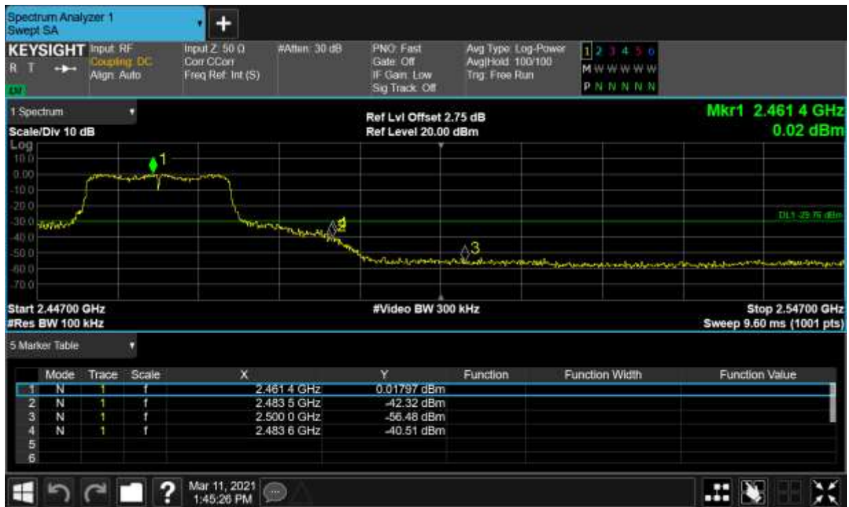
Band Edge NVNT n20 2462MHz Ant2 Ref
