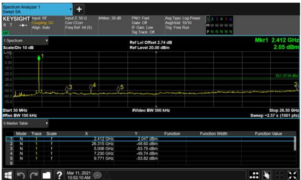
Tx. Spurious NVNT g 2437MHz Ant2 Ref
