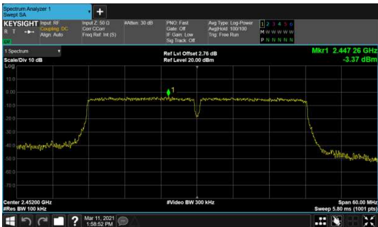
Band Edge NVNT n40 2452MHz Ant2 Emission
