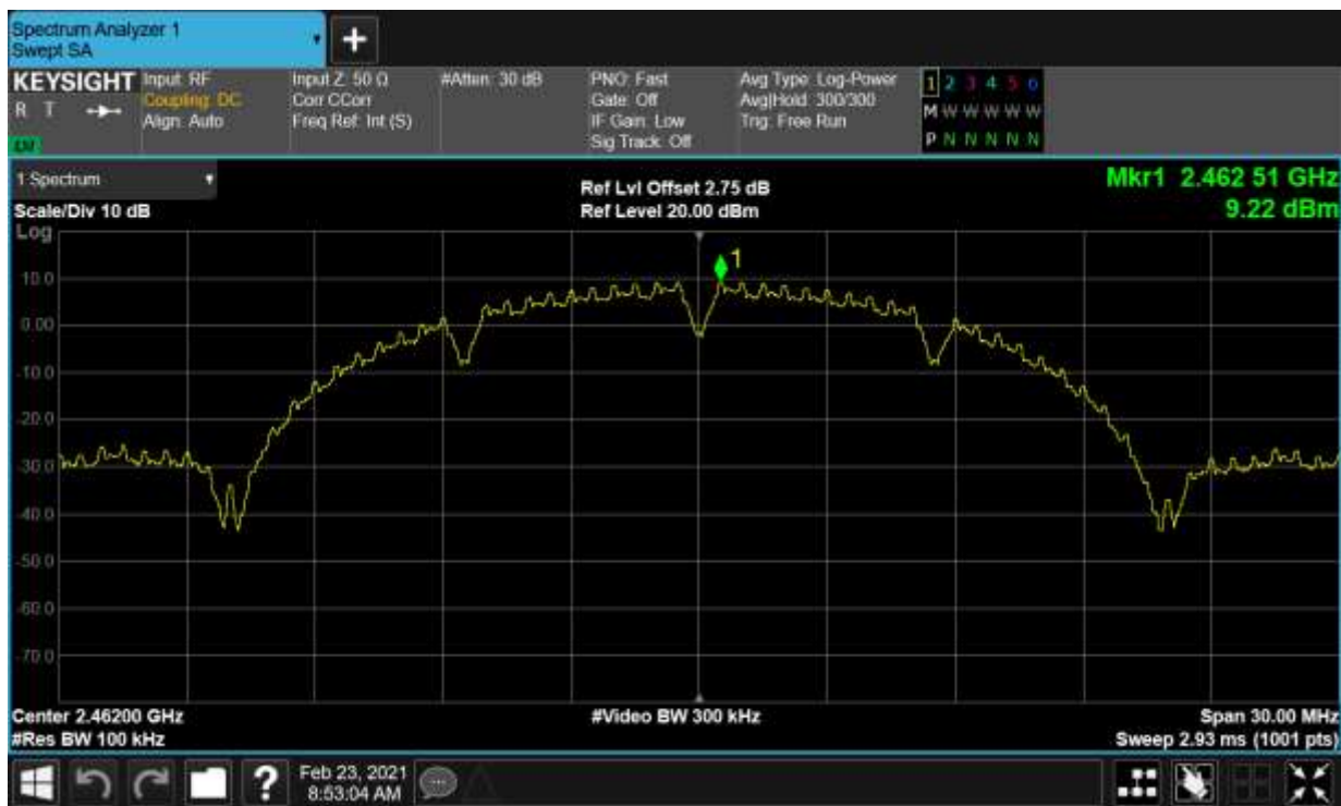
Band Edge NVNT b 2462MHz Ant1 Emission
