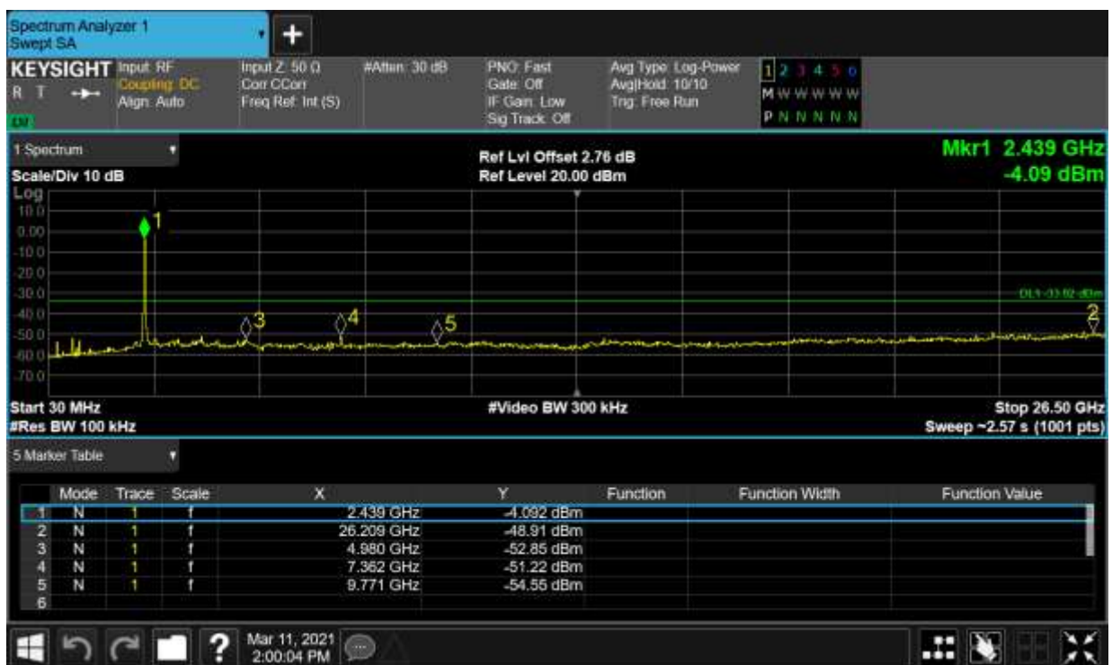
Tx. Spurious NVNT n40 2452MHz Ant2 Emission
