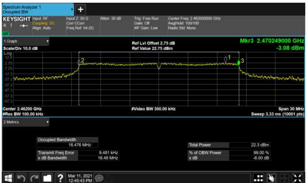
-6dB Bandwidth NVNT g 2412MHz Ant2
