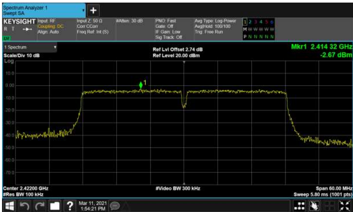
Band Edge NVNT n40 2422MHz Ant2 Emission
