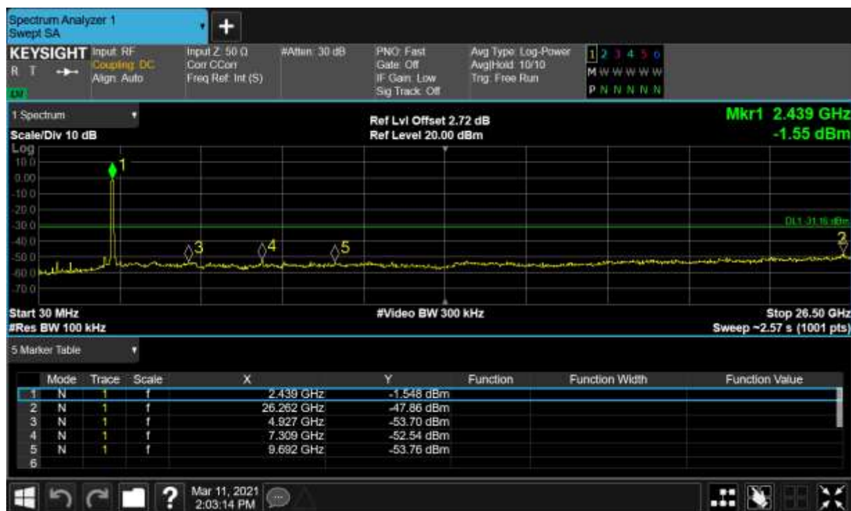
Tx. Spurious NVNT n40 2437MHz Ant2 Ref
