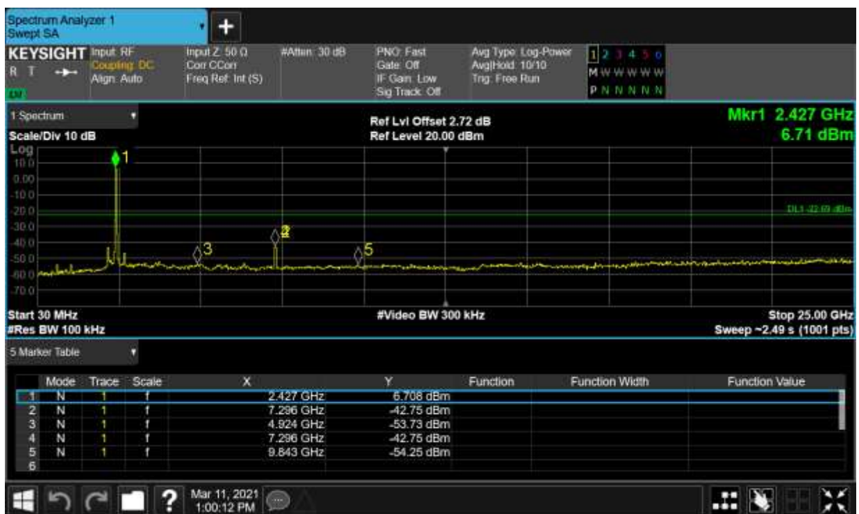
Tx. Spurious NVNT g 2462MHz Ant1 Ref
