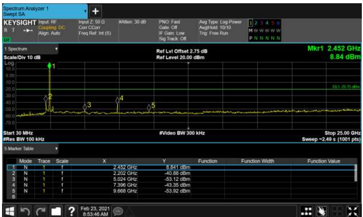
Tx. Spurious NVNT b 2412MHz Ant2 Ref
