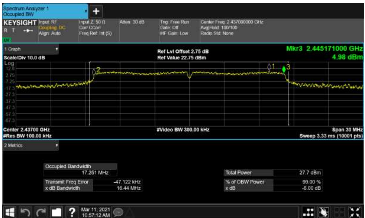
-6dB Bandwidth NVNT g 2462MHz Ant2
