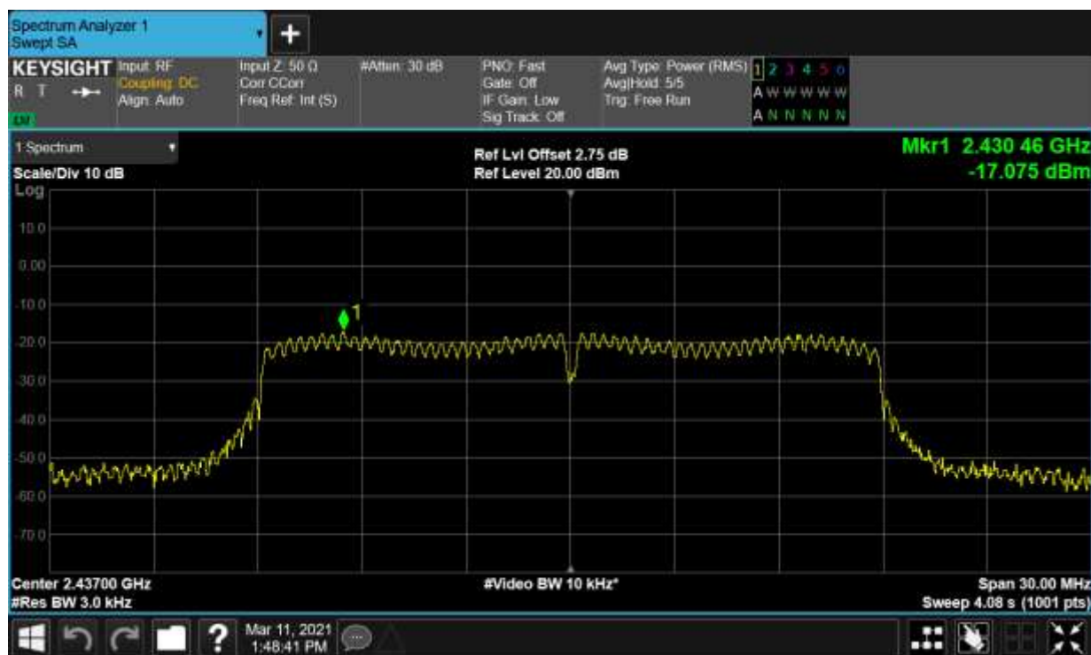
PSD NVNT n20 2462MHz Ant1
