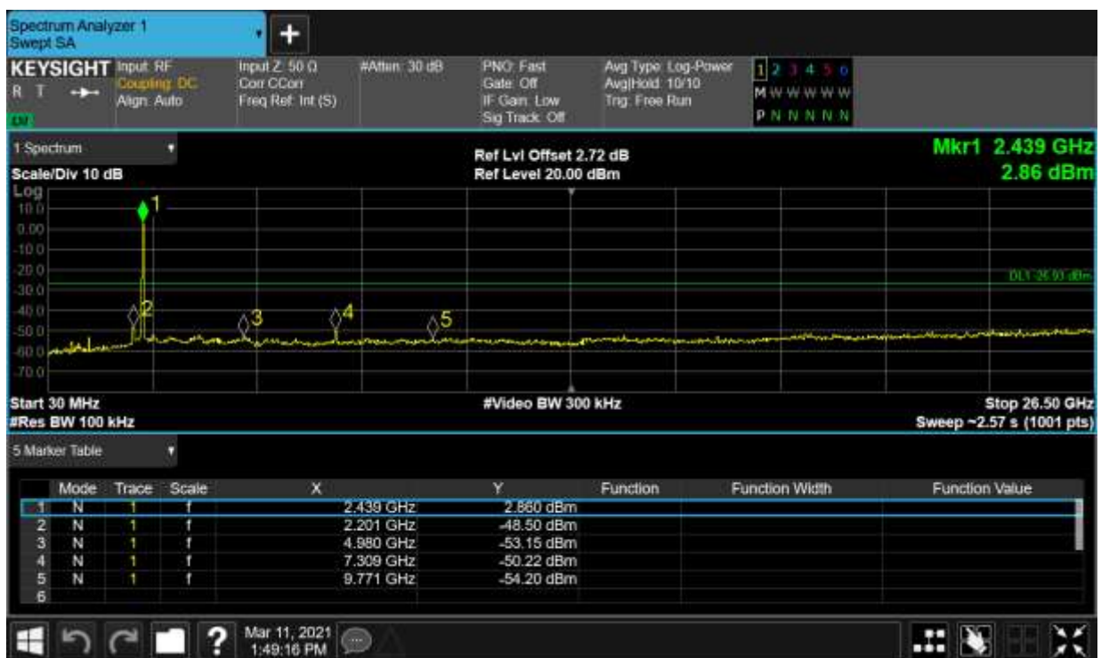
Tx. Spurious NVNT n20 2437MHz Ant2 Ref
