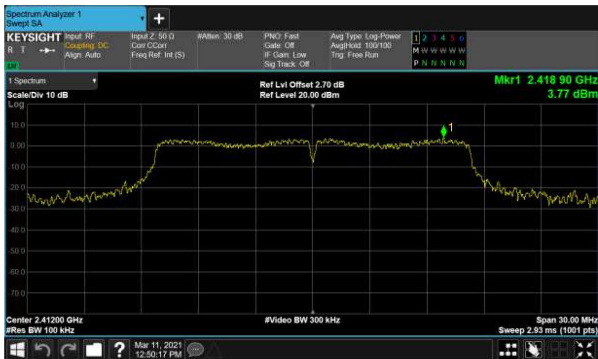
Tx. Spurious NVNT g 2412MHz Ant1 Emission
