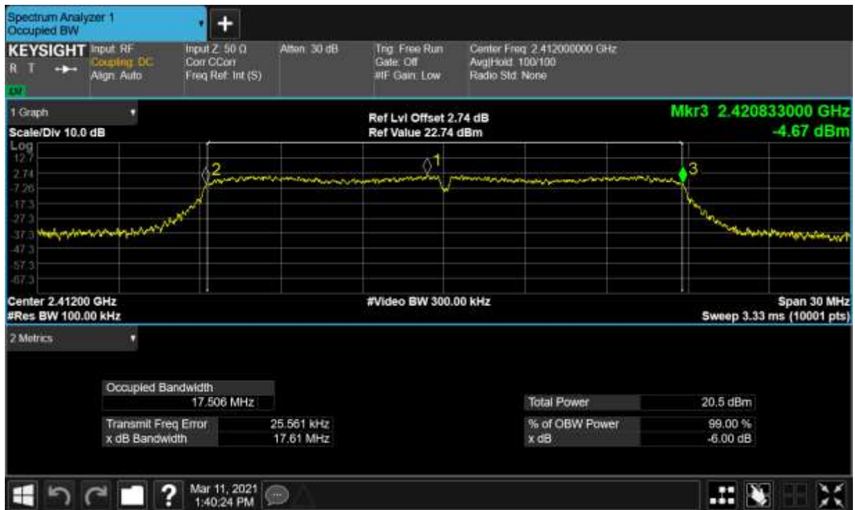
-6dB Bandwidth NVNT n20 2437MHz Ant1
