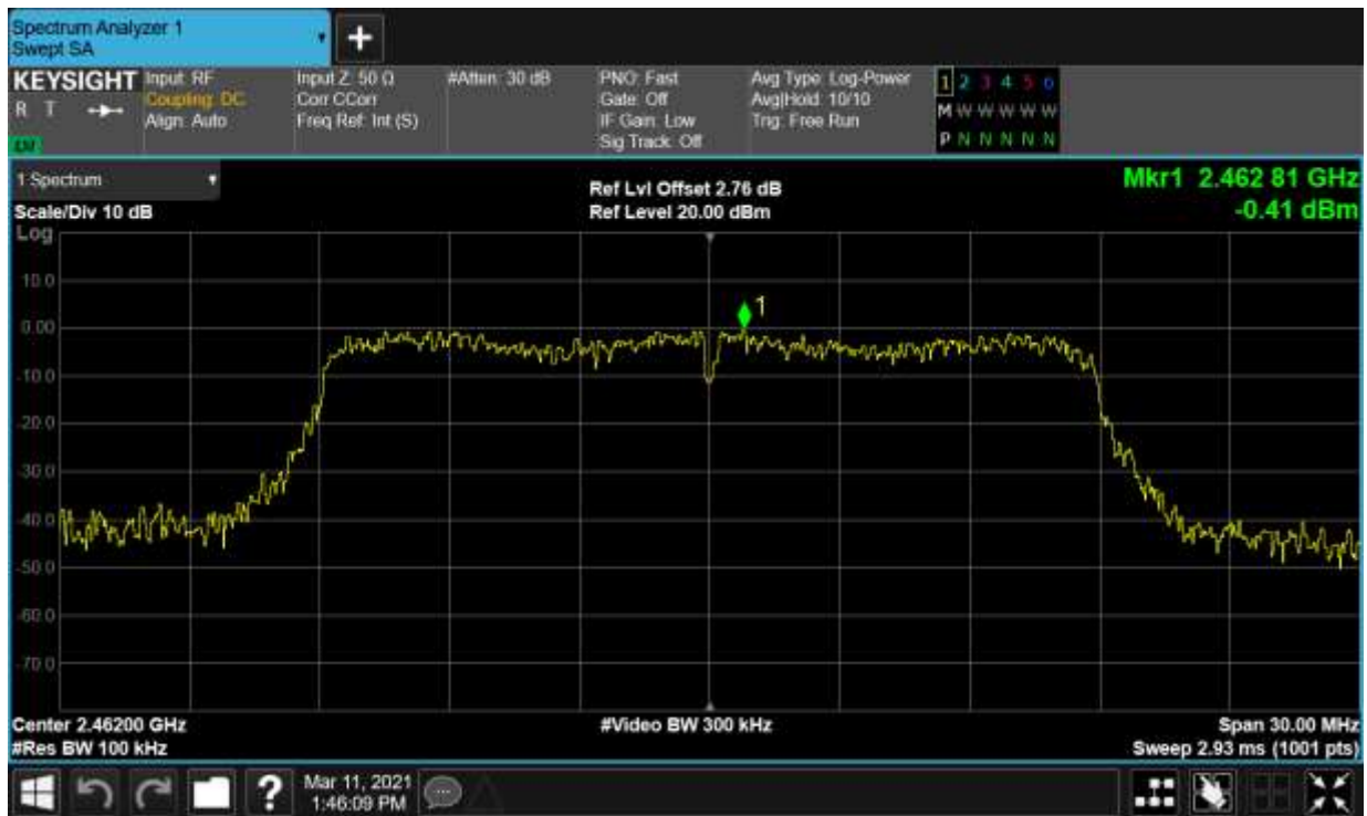
Tx. Spurious NVNT n20 2462MHz Ant2 Emission
