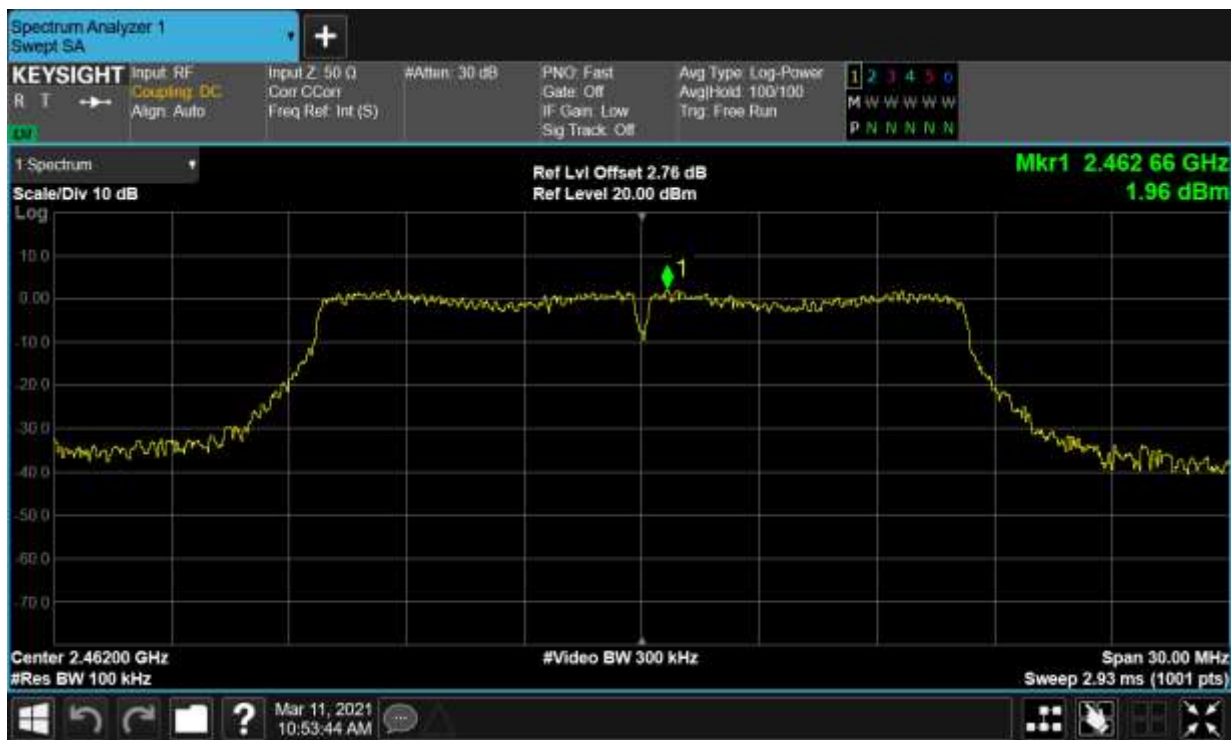
Band Edge NVNT g 2462MHz Ant2 Emission
