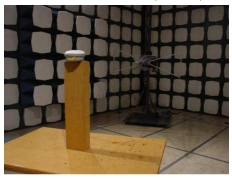
RADIATED SPURIOUS EMISSION TEST (ABOVE 1GHZ)
