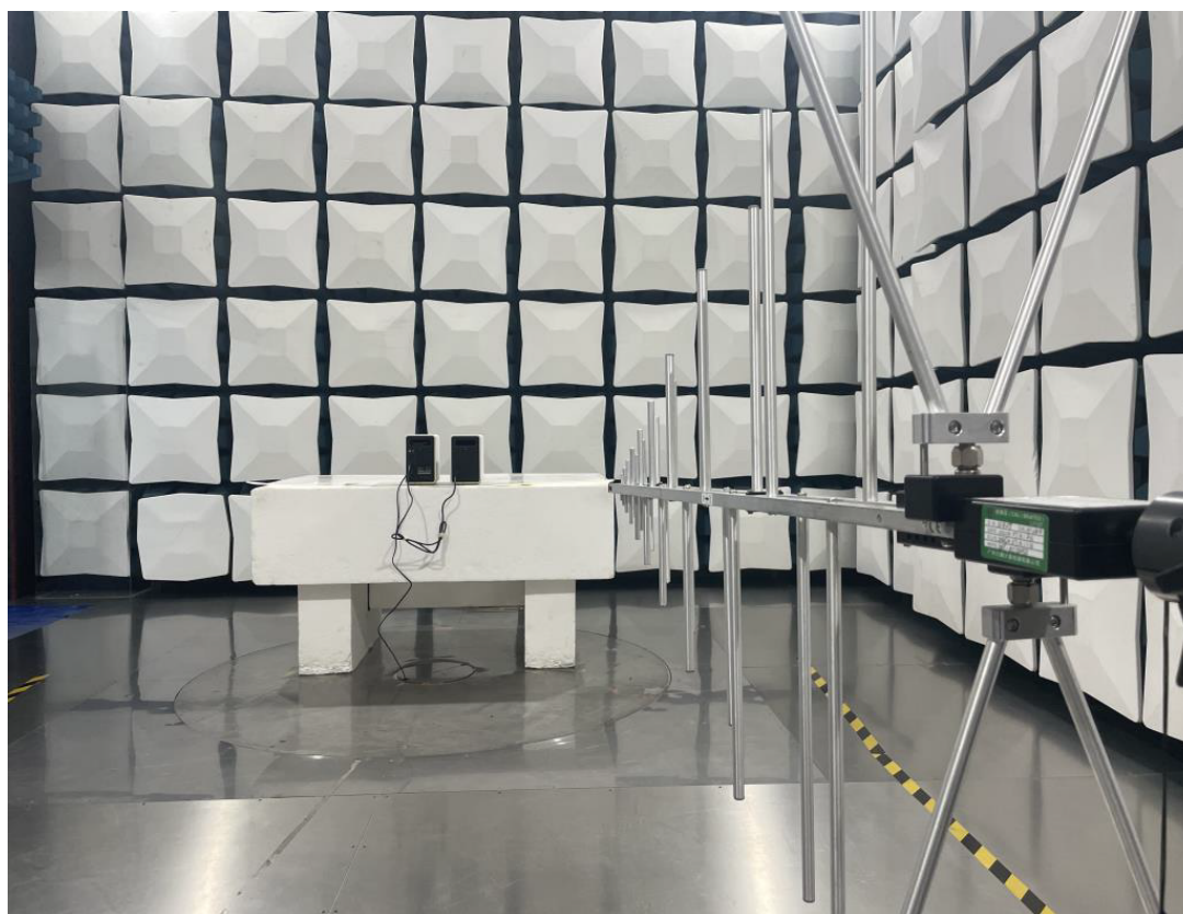
Photograph 2: Set-up for Radiated Spurious Emission, 30MHz - 1GHz
