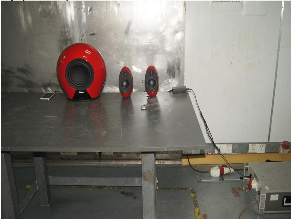
Photograph 2: Set-up for Spurious Emissions for below 30MHz
