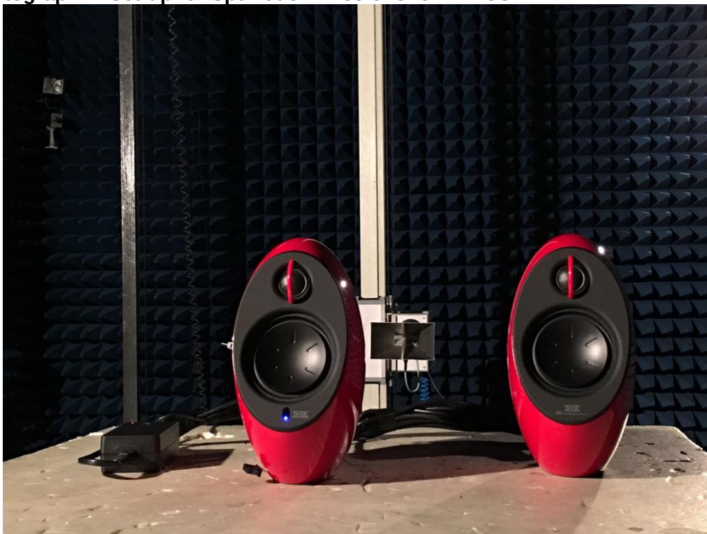
Photograph 4: Set-up for Spurious Emissions for 1 - 18GHz
