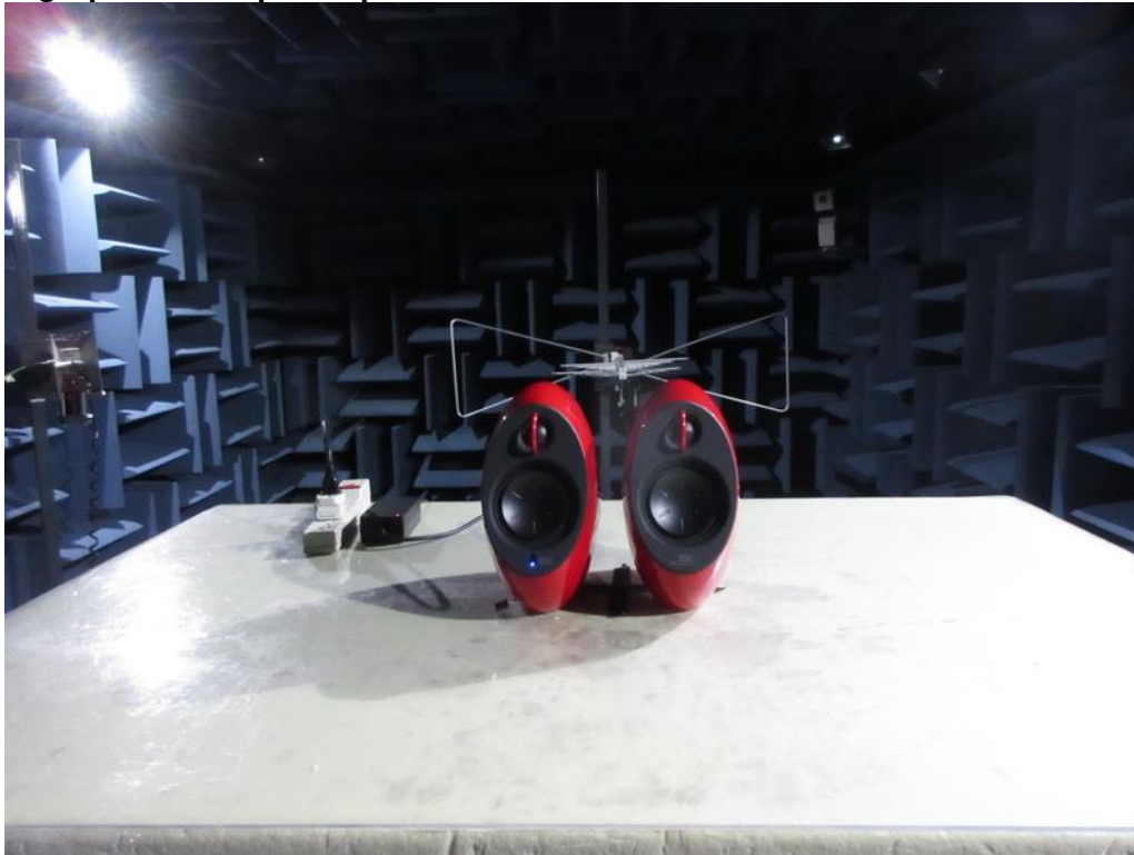
Photograph 4: Set-up for Spurious Emissions for 1 - 18GHz
