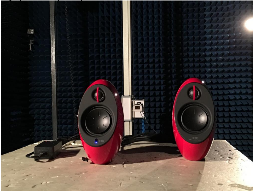
Photograph 6: Set-up for Spurious Emissions for 26.5 - 40GHz
