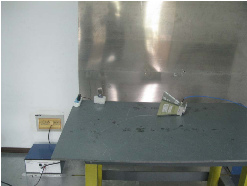
Conducted Emissions Test Setup Front View
