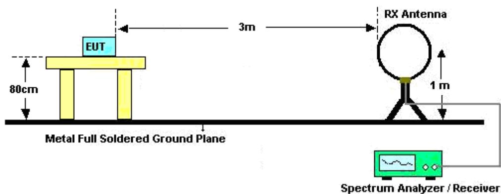
For radiated emissions from 30MHz to 1GHz
