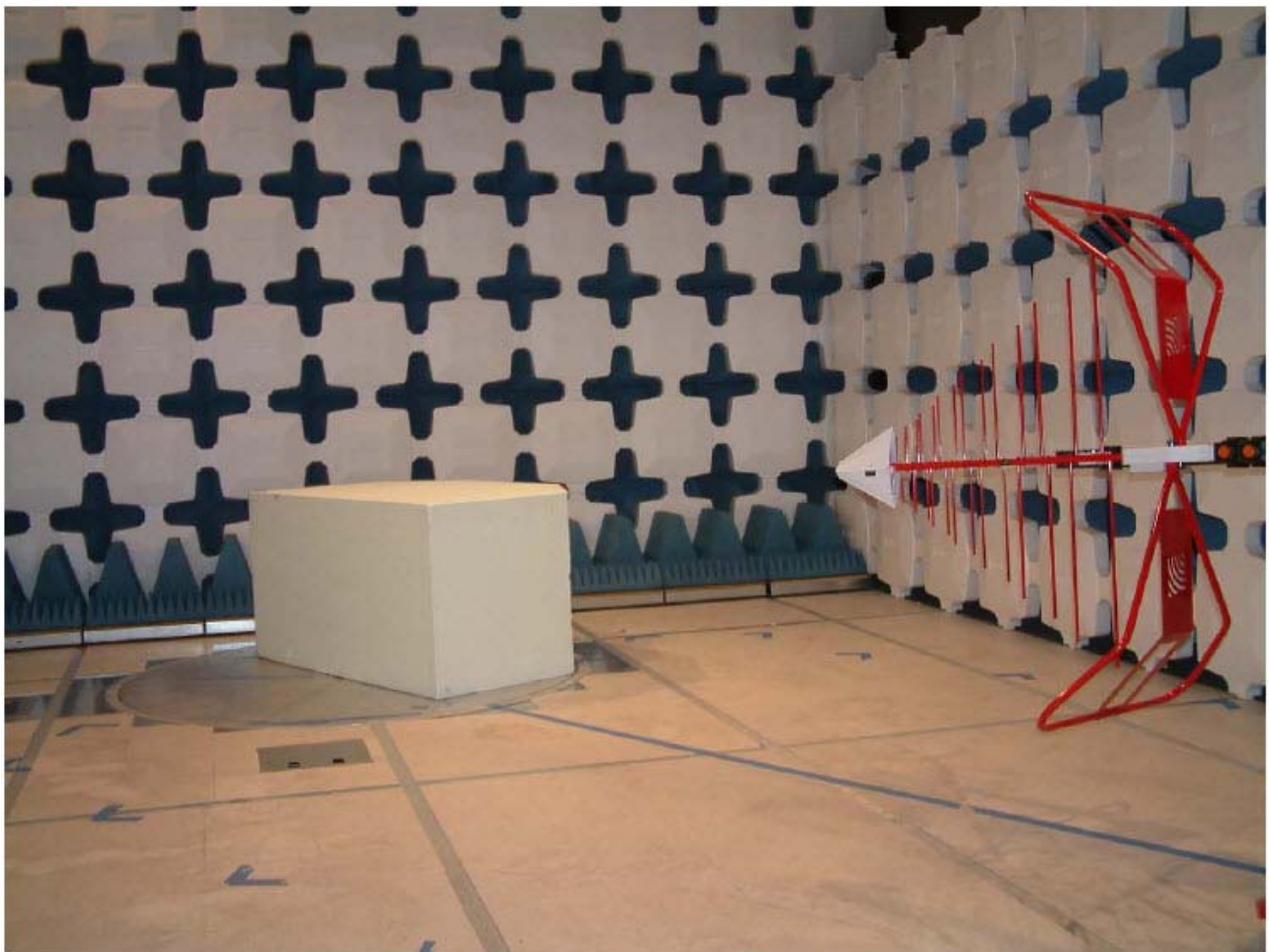
Figure 3.1 – Test Facility (setup for 30 MHz – 1GHz)
