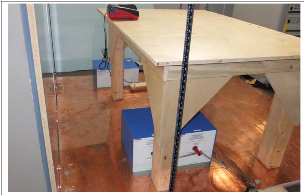
Figure 3.6- Conducted Emissions test setup
