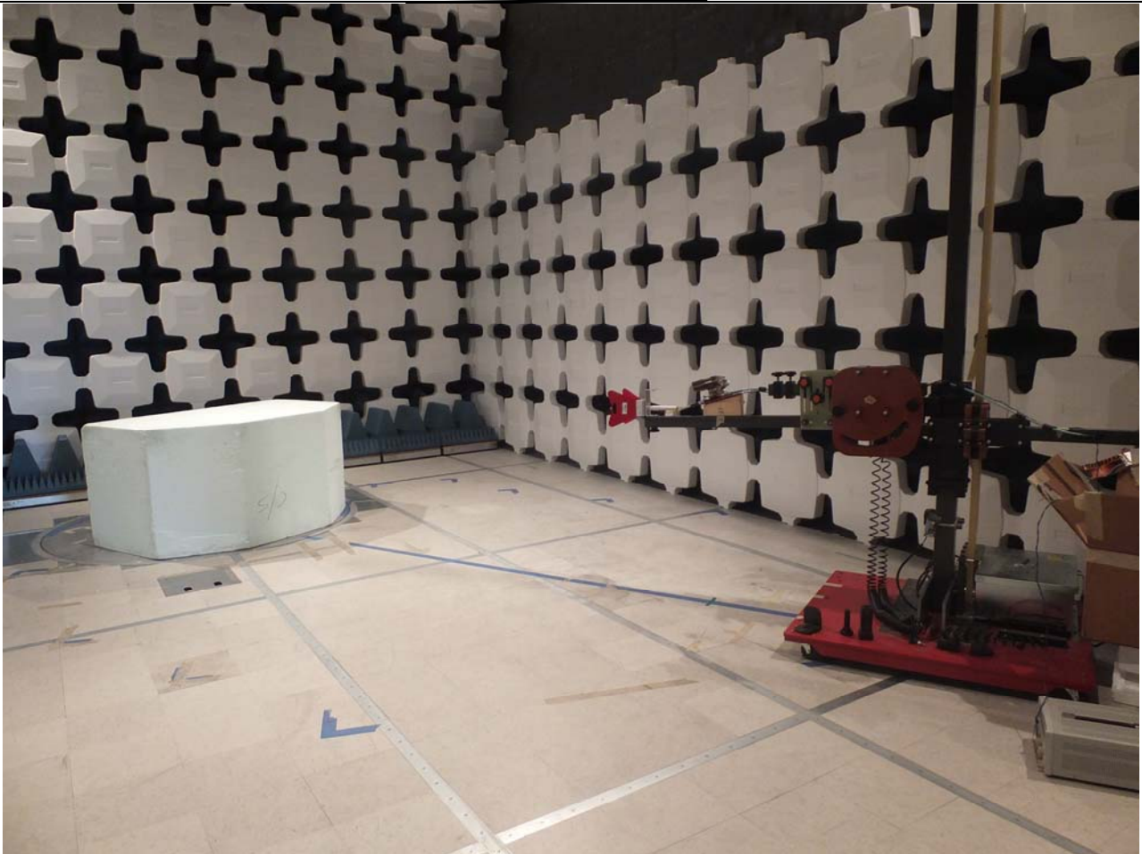
Figure 3.2 – Test Facility (setup for 1 GHz – 18 GHz)
