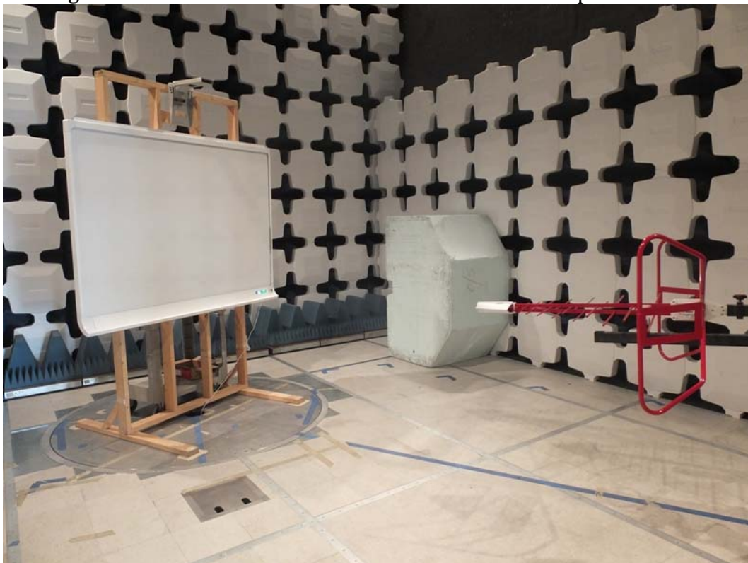
Figure 4.4B – Radiated Emissions 30M-1000M Test Setup - Side View
