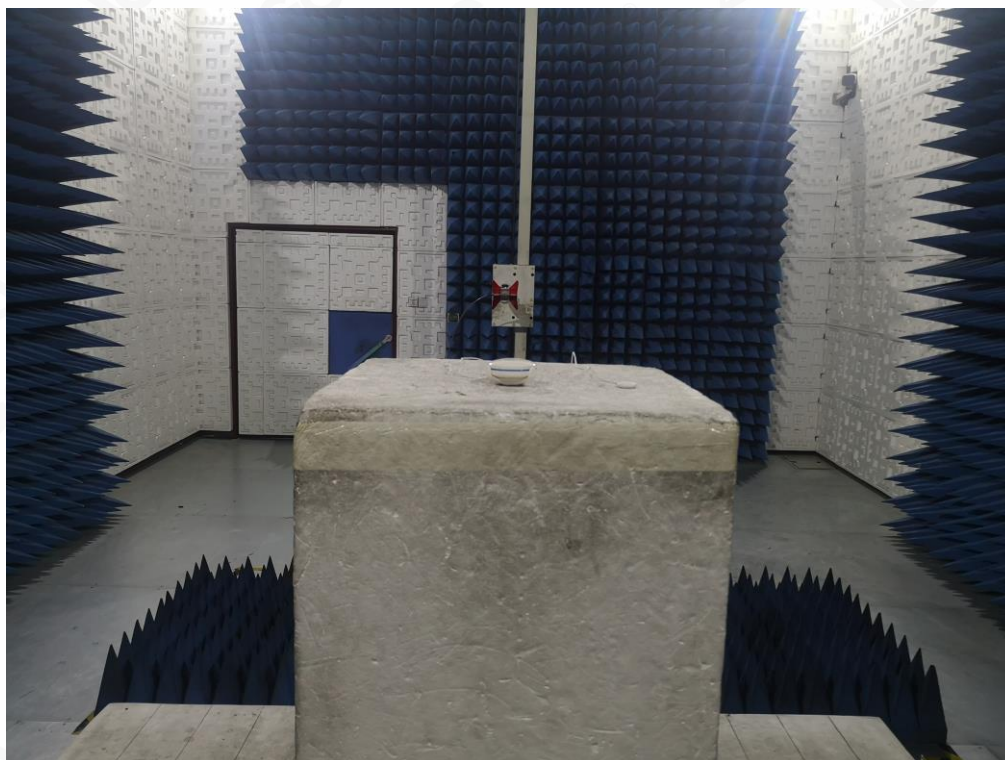
FCC RADIATED EMISSION TEST SETUP ABOVE 1GHZ
