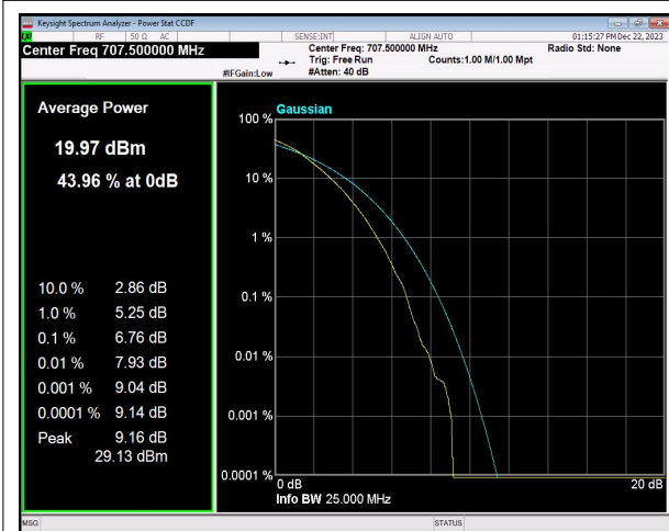
n12 SCS=15kHz DFT_256QAM BW=15MHz Channel=141500 RB=75@0
