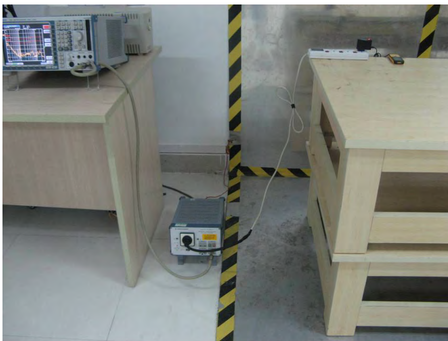
CONDUCTED EMISSION TEST SETUP
