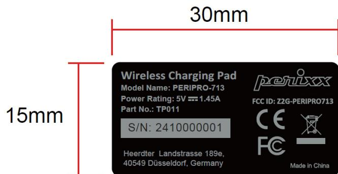
Specifications: Text is Black in color and justified. Labels are printed in indelible ink on permanent adhesive or silk-screened onto the EUT or shall be affixed at a conspicuous location on the EUT.
