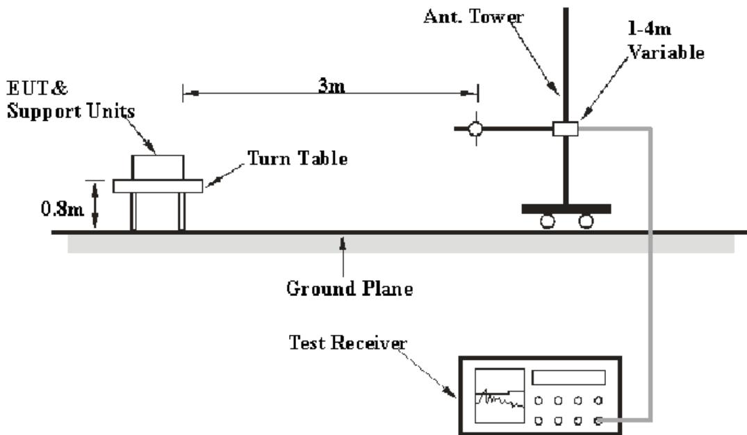
The deactivation test was performed in the 3 meters chamber test site, using the setup accordance with the ANSI C63.4 - 2009. The specification used was the FCC 15.231(e) limits.
