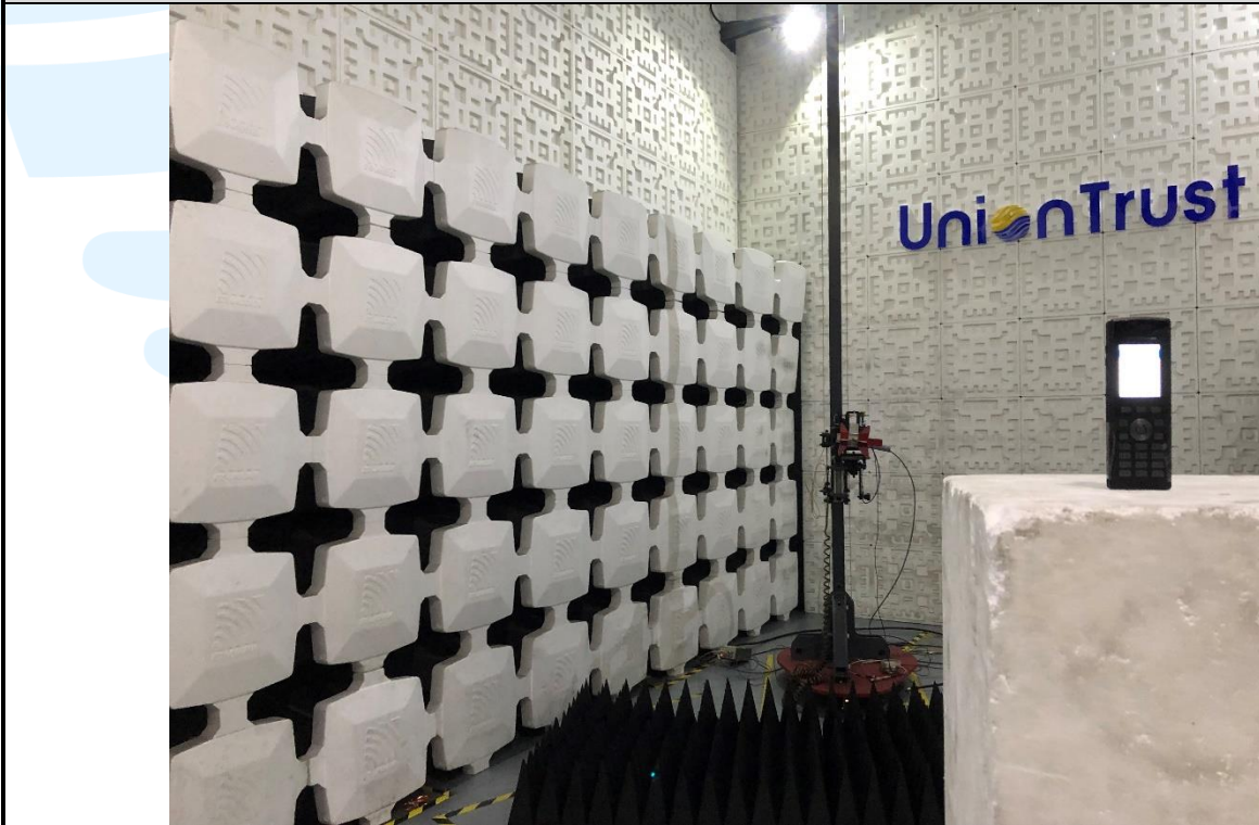
Radiated emission Test Setup (Above 1 GHz)
