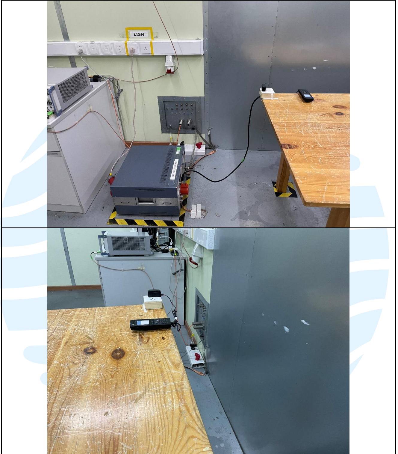
Conducted Emission Test Setup-3
