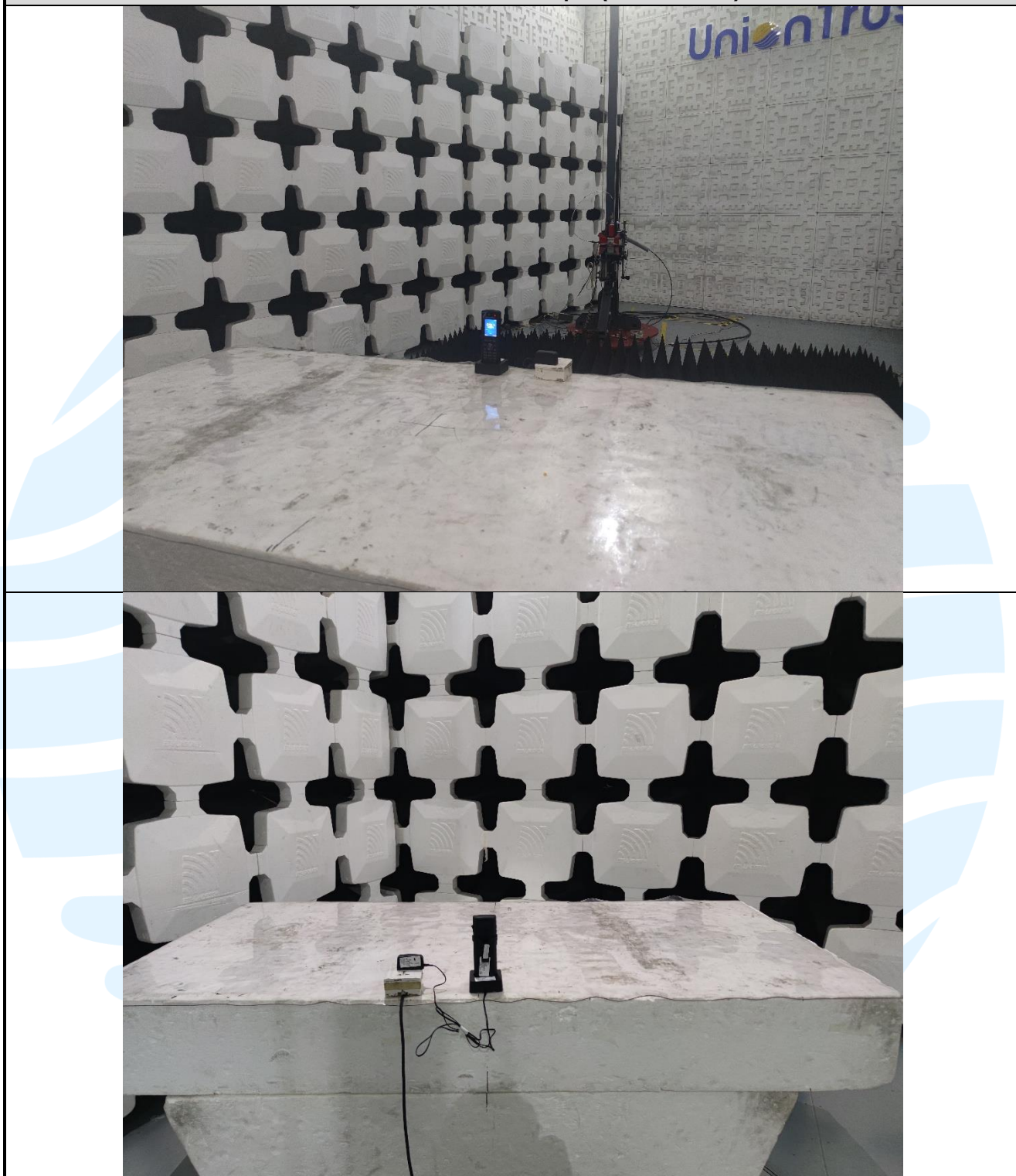
Radiated emission Test Setup-2 (Above 1 GHz)
