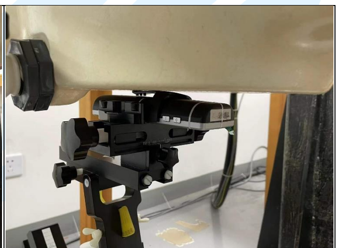
Rear Face of EUT with 0 cm Gap with Belt Clip
