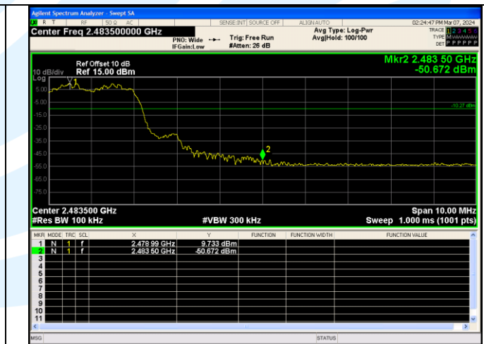
Out Of Band Emission(Right) 8DPSK_3-DH5_Channel Hopping
