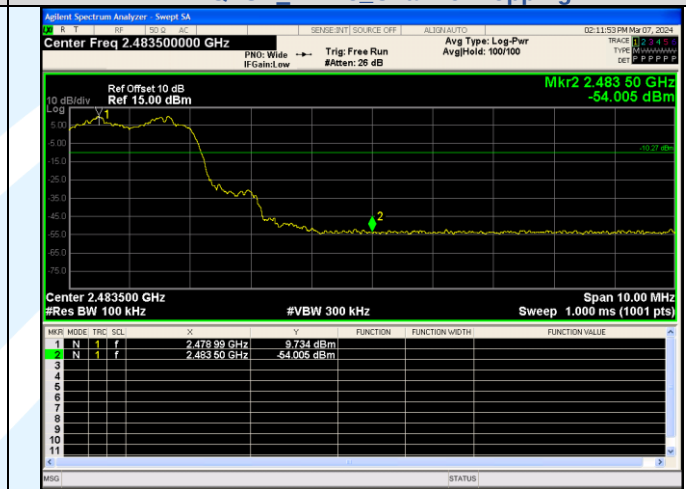
Out Of Band Emission(Right) \pi/4 DQPSK_2-DH5_Channel Hopping
