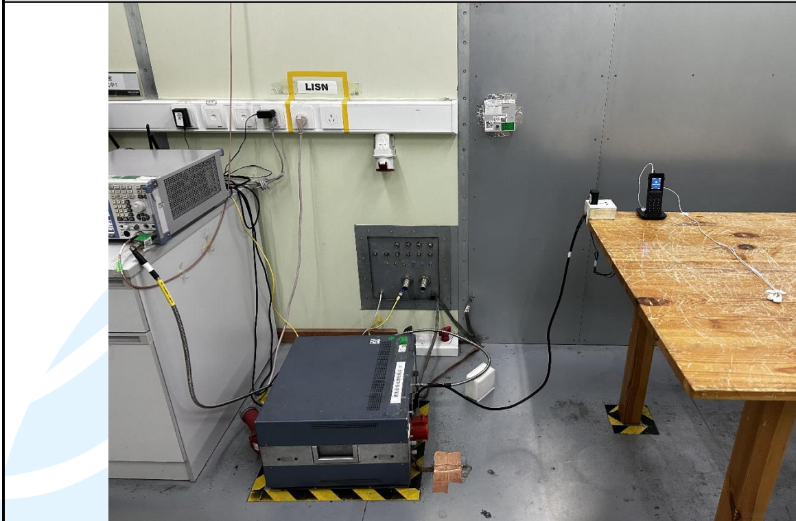
Conducted Emission Test Setup
