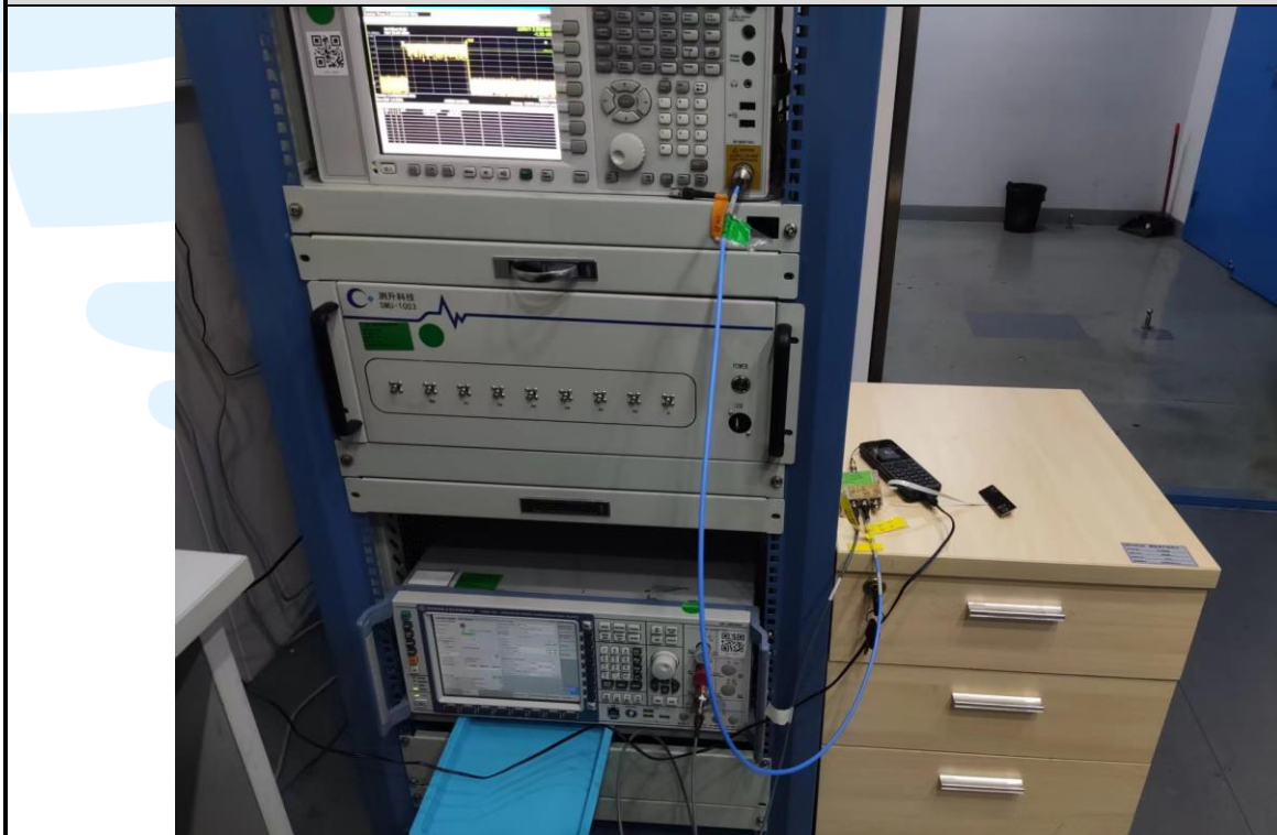
RF Conducted Test Setup
