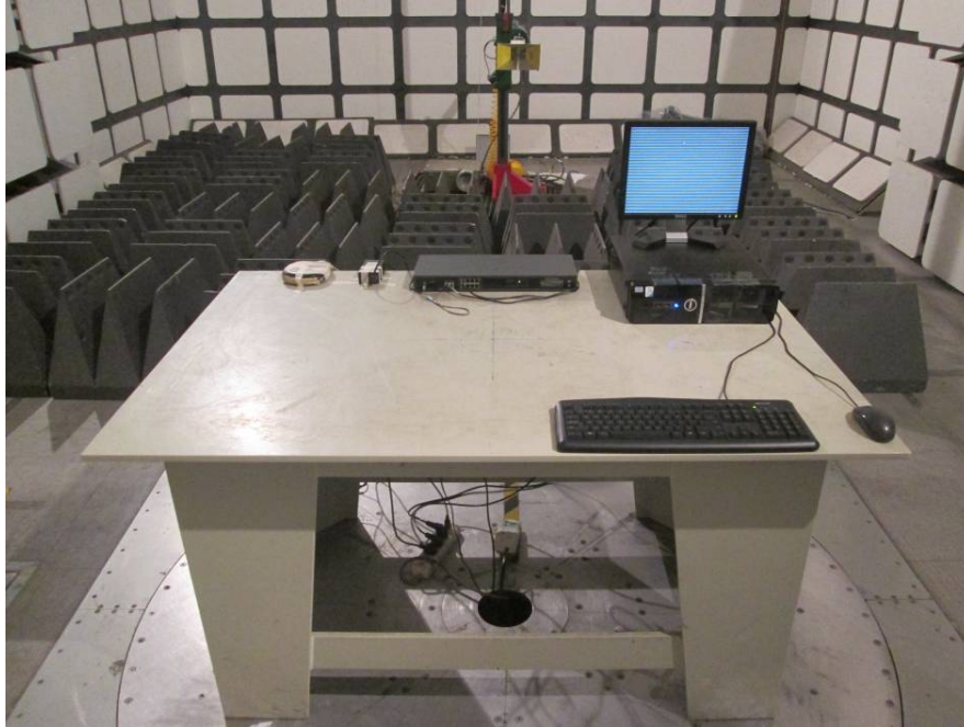
Radiated Emissions Front View (Below 1 GHz, Power by POE)
