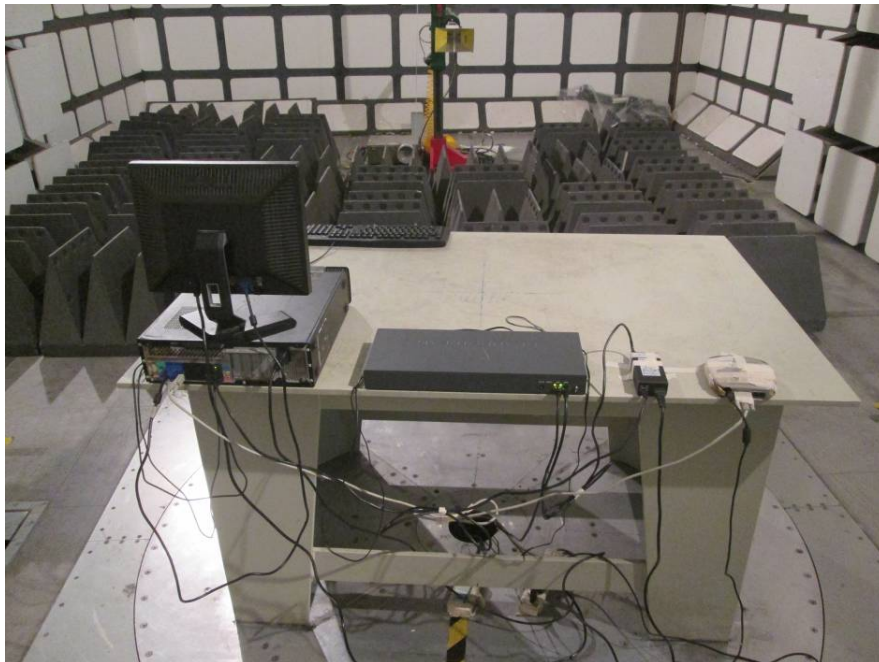
Radiated Emissions Rear View (Below 1 GHz, Power by POE)
