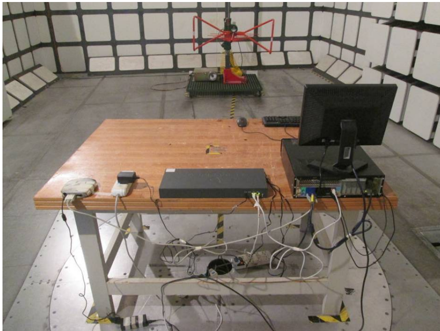
Radiated Emissions Rear View (Below 1 GHz, Power by adapter)
