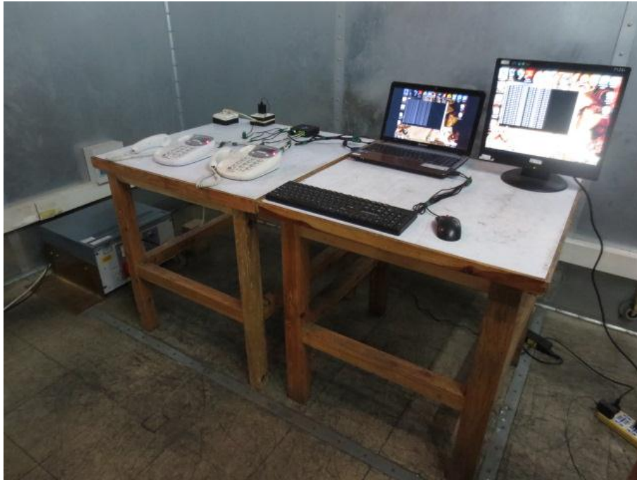
Conducted Emission Test Set-up -Front view
