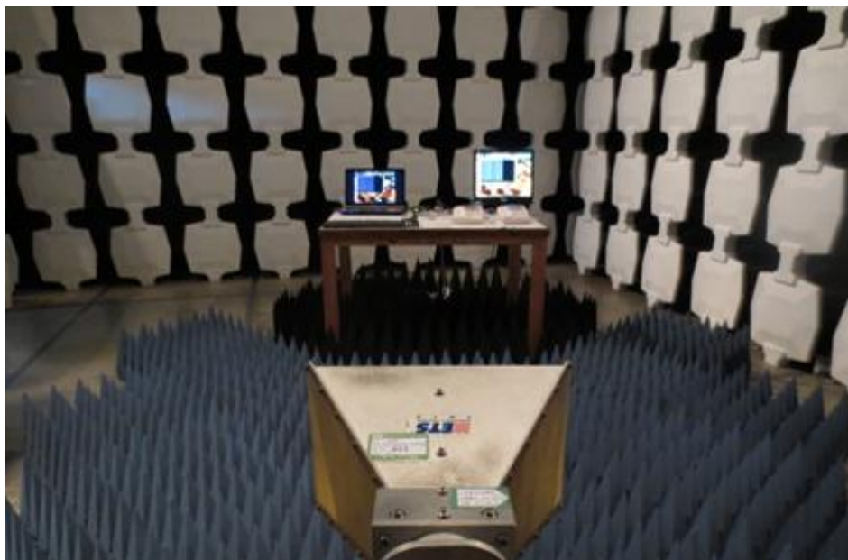
Radiated Emission Test Set-up(Above 1GHz)
