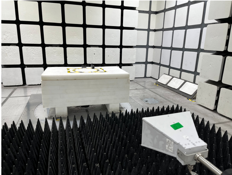
Radiated Emissions Front View (Above 1 GHz)
