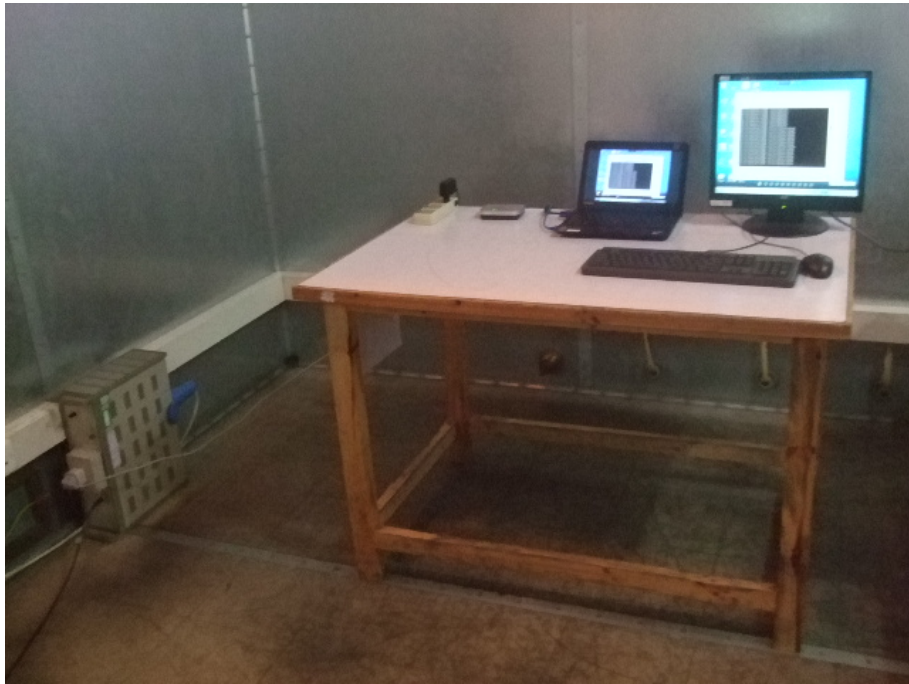
Conducted Emission Test Set-up (front view)
