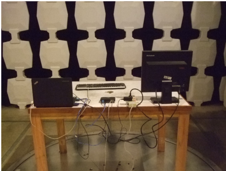
Radiated Emission Test Set-up (rear view)
