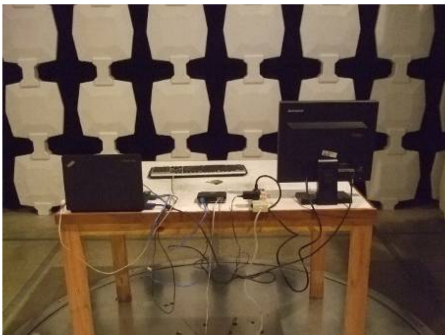
Radiated Emission Test Set-up (rear view)
