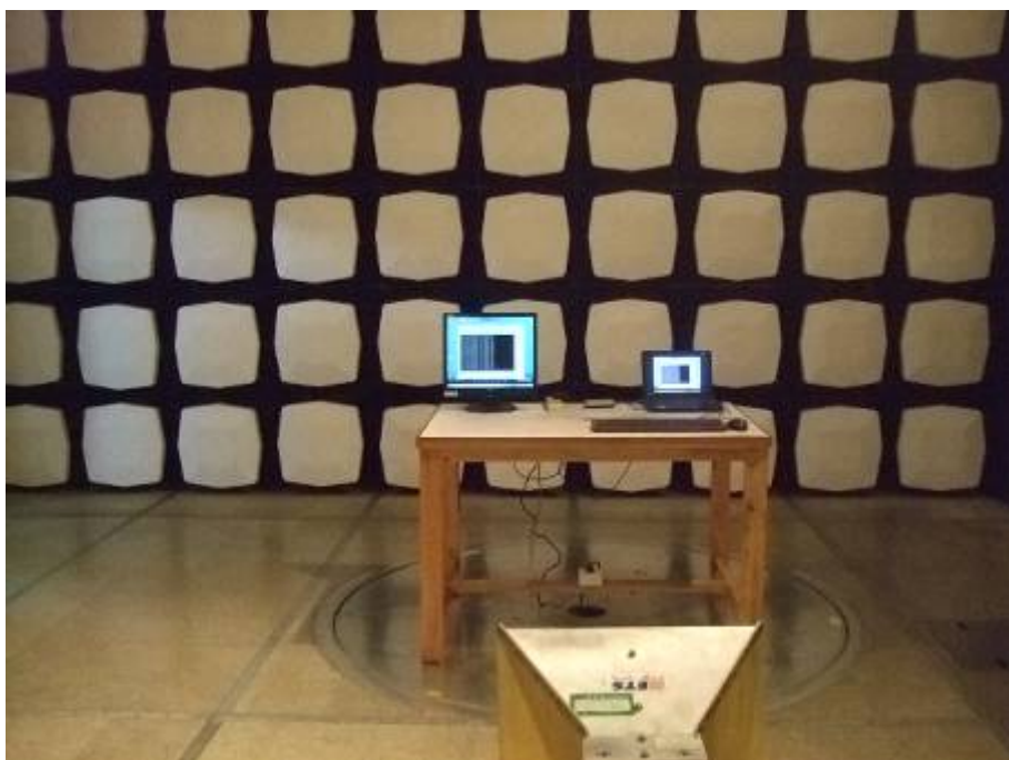
Radiated Emission Test Set-up (Above 1GHz)
