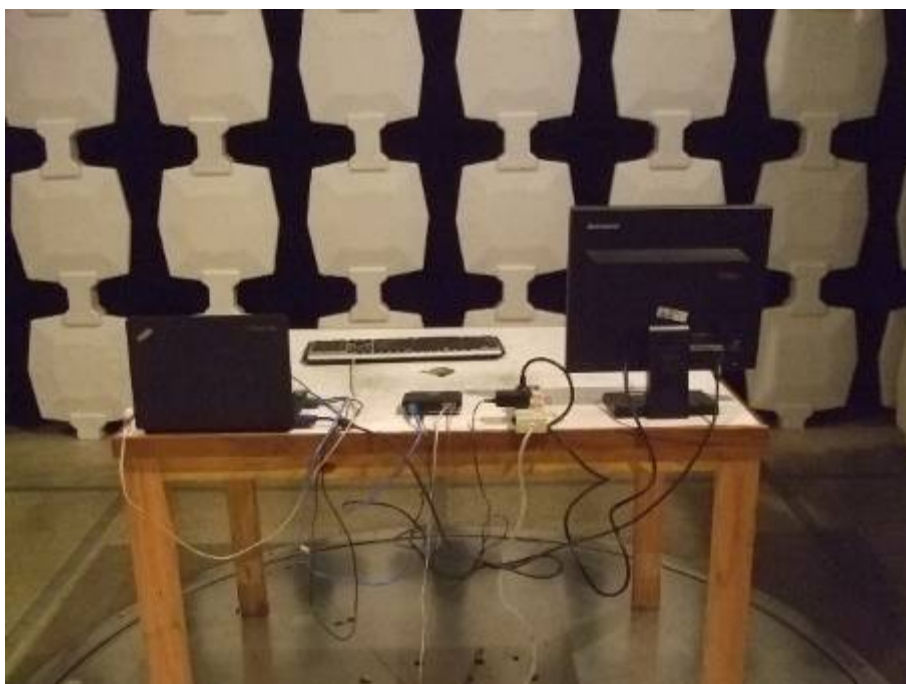
Radiated Emission Test Set-up (rear view)
