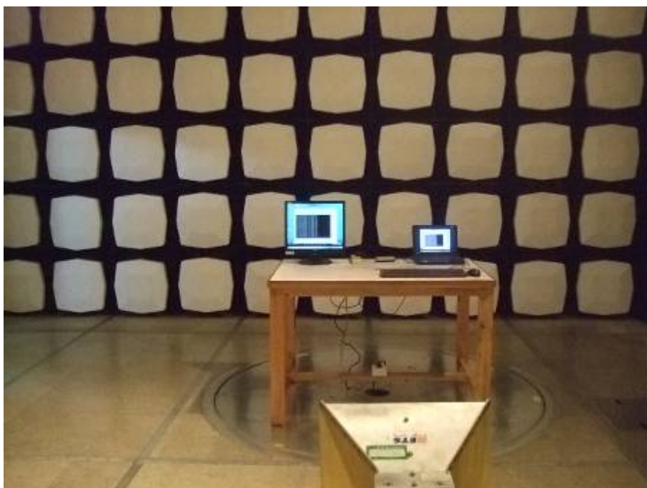
Radiated Emission Test Set-up (Above 1GHz)
