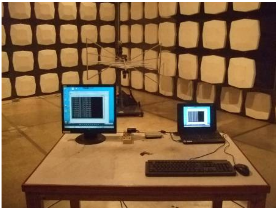
Radiated Emission Test Set-up (Below 1GHz)
