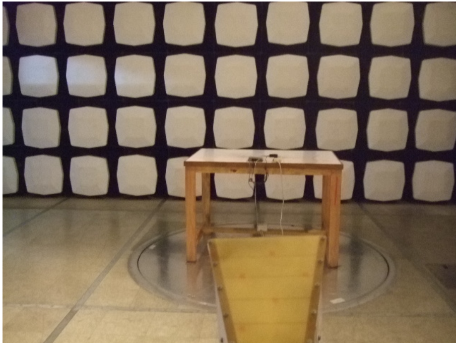
IP Call:Radiated Emission Test Set-up(Above 1GHz)
