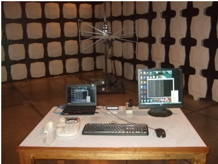
Radiated Emission Test Set-up (Below 1GHz)
