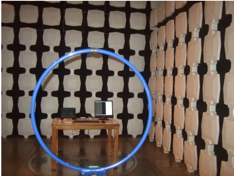
Radiated Emission Test Set-up (9KHz-30MHz)
