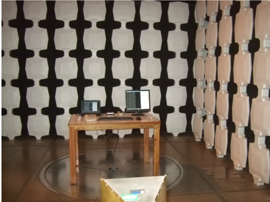
Radiated Emission Test Set-up (Above 1GHz)
