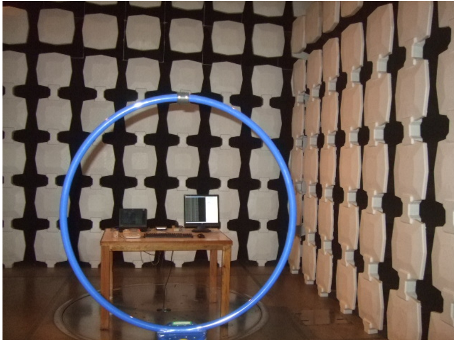
Radiated Emission Test Set-up (9KHz-30MHz)
