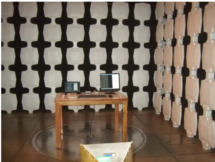
Radiated Emission Test Set-up (Above 1GHz)
