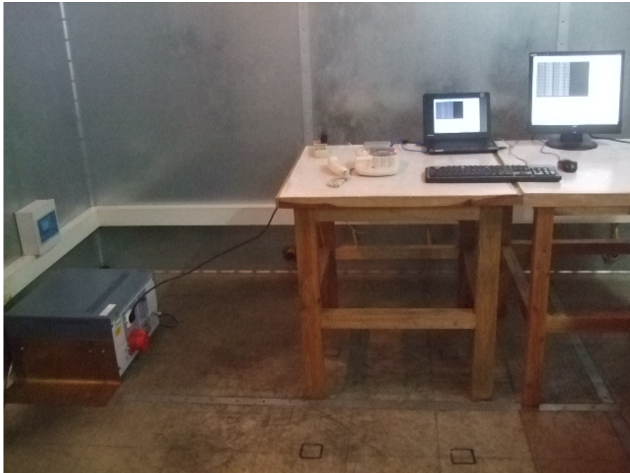
Conducted Emission Test Set-up -front view
