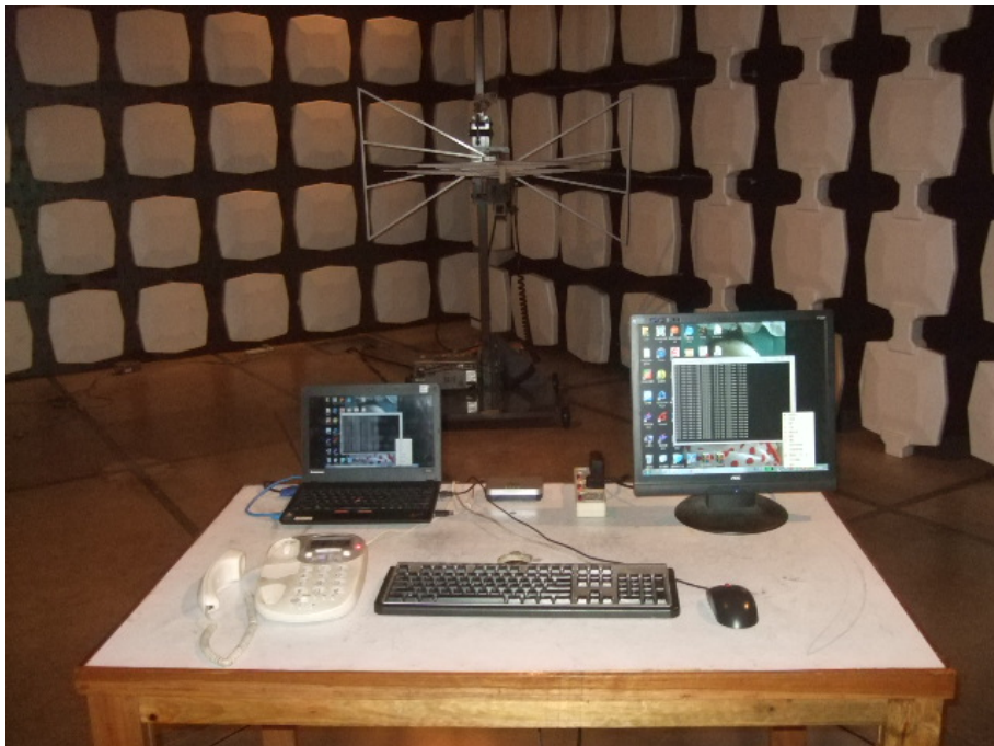
Radiated Emission Test Set-up (Below 1GHz)
