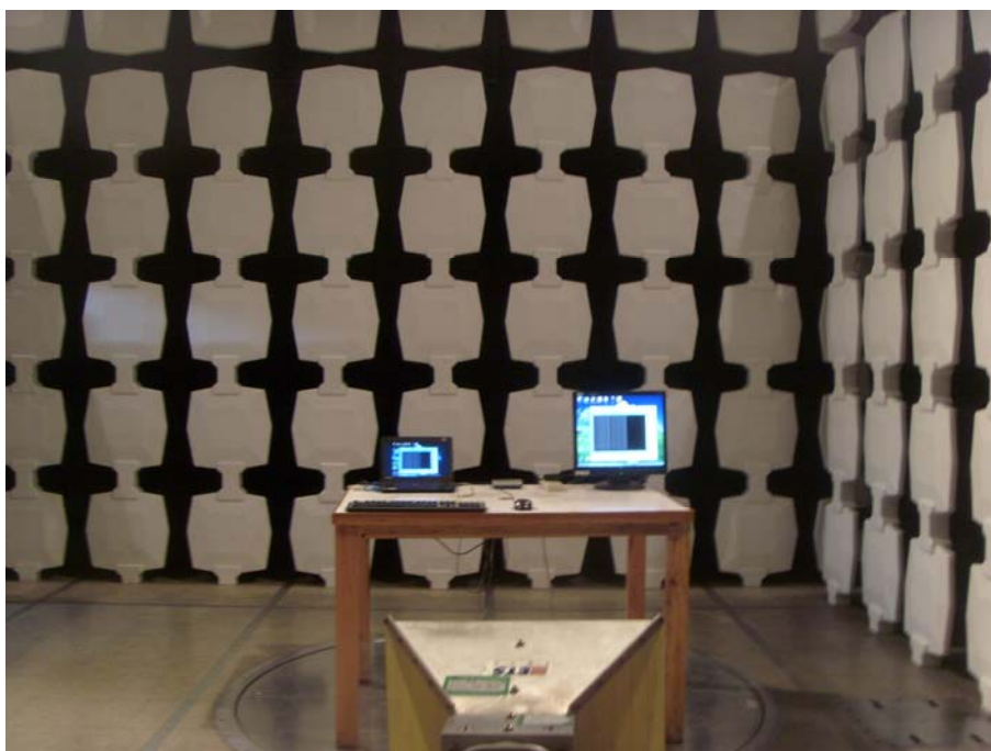
Radiated Emission Test Set-up (Above 1GHz)
