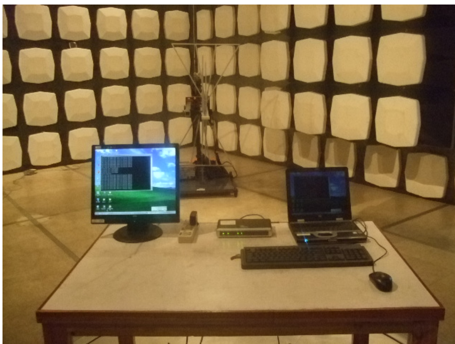
Radiated Emission Test Set-up(30MHz- 1000MHz)
