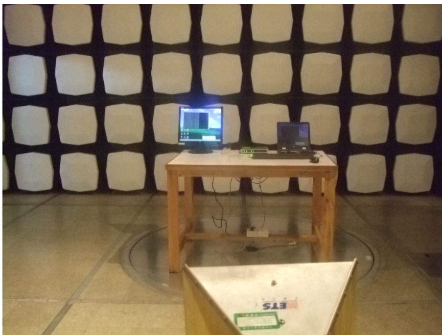
Radiated Emission Test Set-up(Above 1GHz)
