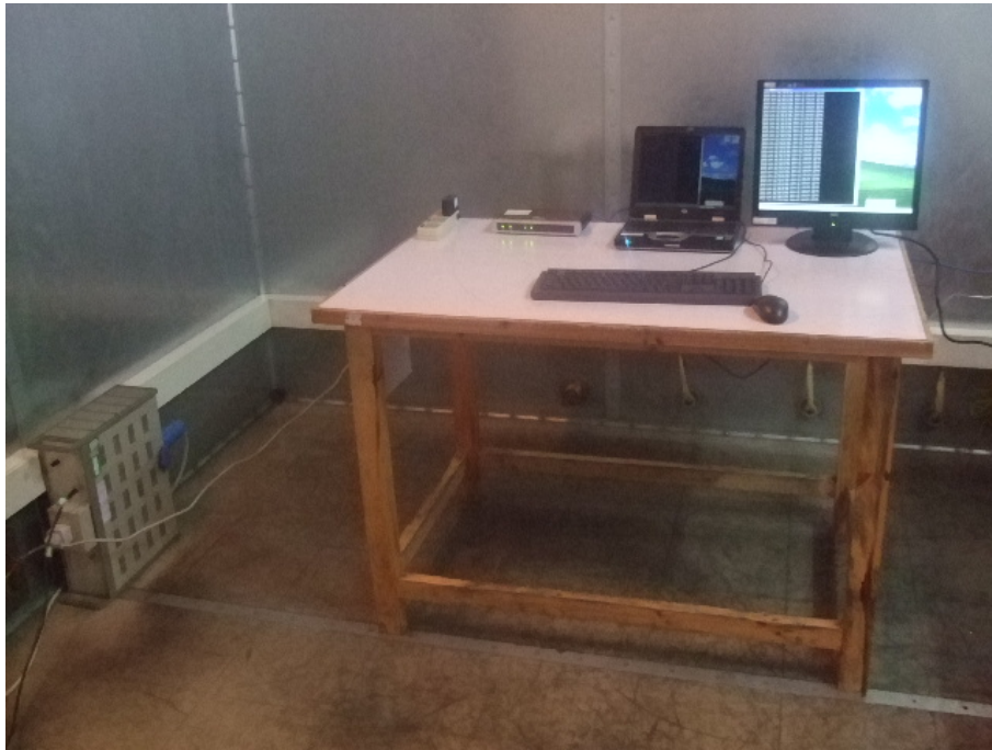
Conducted Emission Test Set-up
