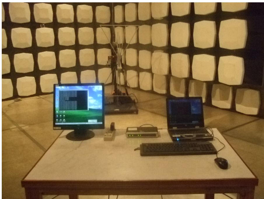
Radiated Emission Test Set-up(30MHz- 1000MHz)
