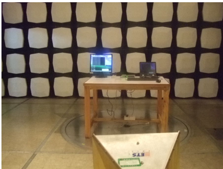
Radiated Emission Test Set-up(Above 1GHz)
