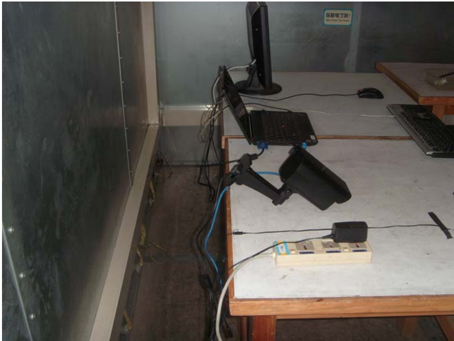
Conducted Emission Test Set-up –Rear view
