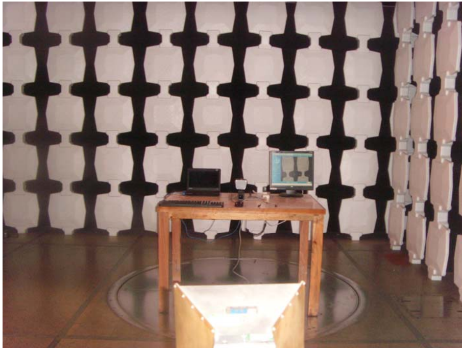
Radiated Emission Test Set-up(Above 1GHz)
