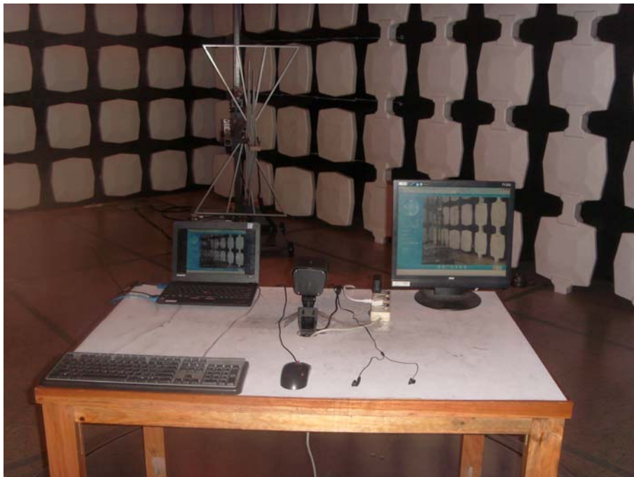
Radiated Emission Test Set-up(Below 1 GHz)
