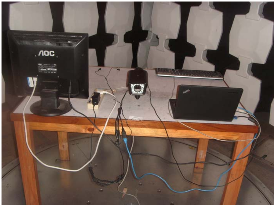
Radiated Emission Test Set-up (Rear view)
