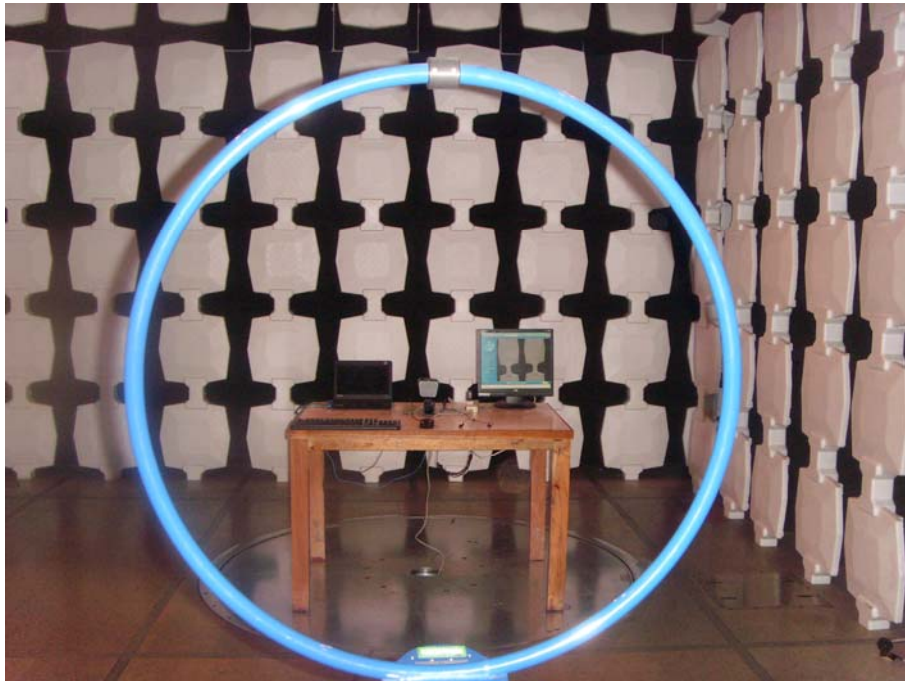
Radiated Emission Test Set-up(9KHz-30MHz)
