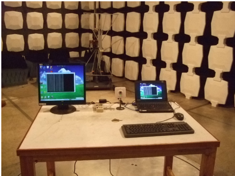
Radiated Emission Test Set-up(Below 1GHz)
