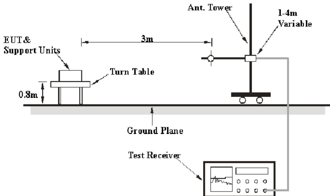
The radiated emission tests were performed in the 3 meters test site, using the setup accordance with the ANSI C63.4-2009. The specification used was the FCC Part 15.109 limits.
