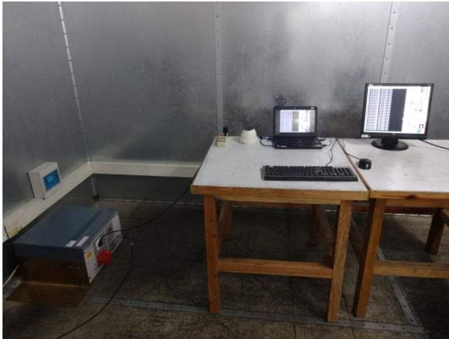
Conducted Emission Test Set-up -Front view
