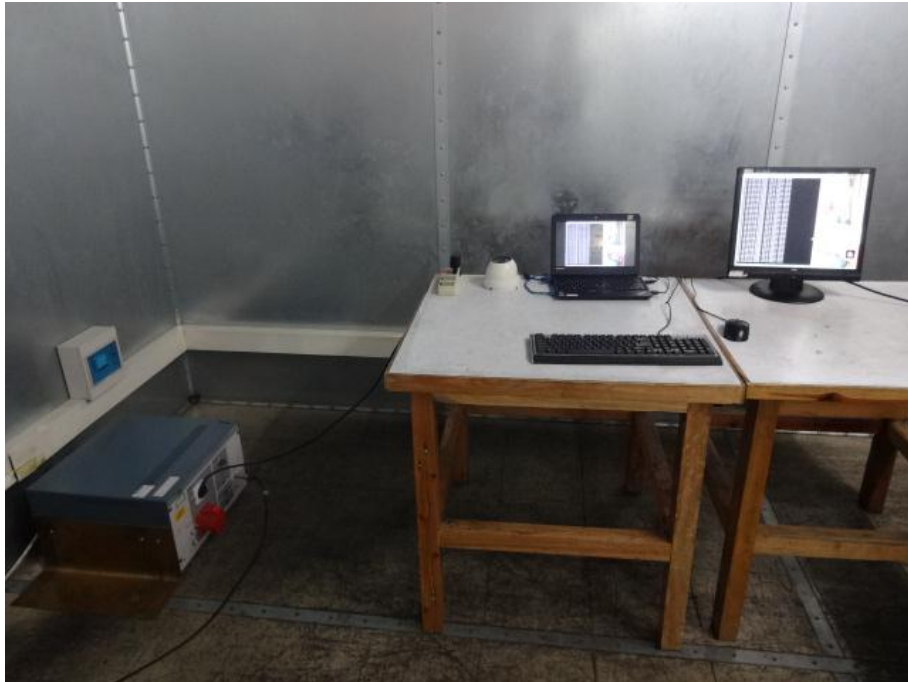
Conducted Emission Test Set-up -Front view
