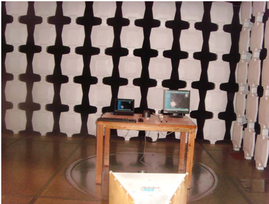
Radiated Emission Test Set-up(Above 1GHz)
