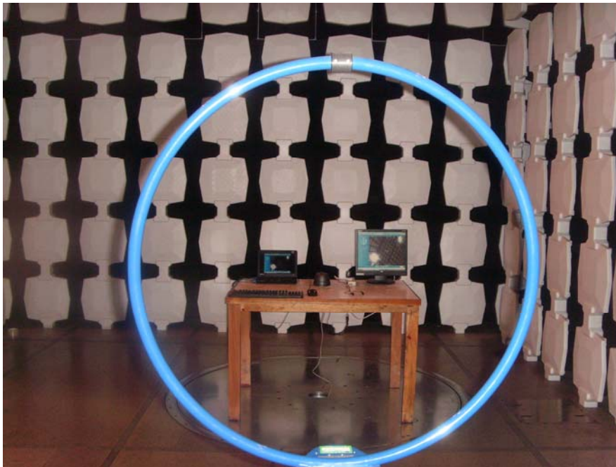
Radiated Emission Test Set-up(9KHz-30MHz)
