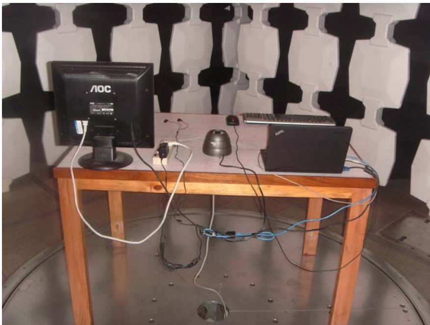
Radiated Emission Test Set-up (Rear View)
