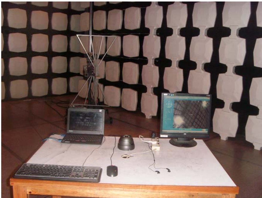
Radiated Emission Test Set-up(Below 1GHz)
