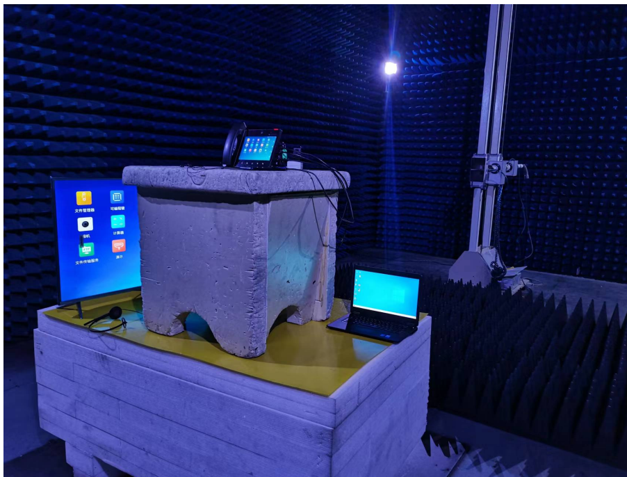
Photo of Radiated Emission Measurement (Above 1G)
