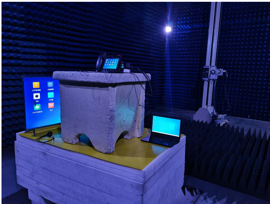
Photo of Radiated Emission Measurement (Above 1G)
