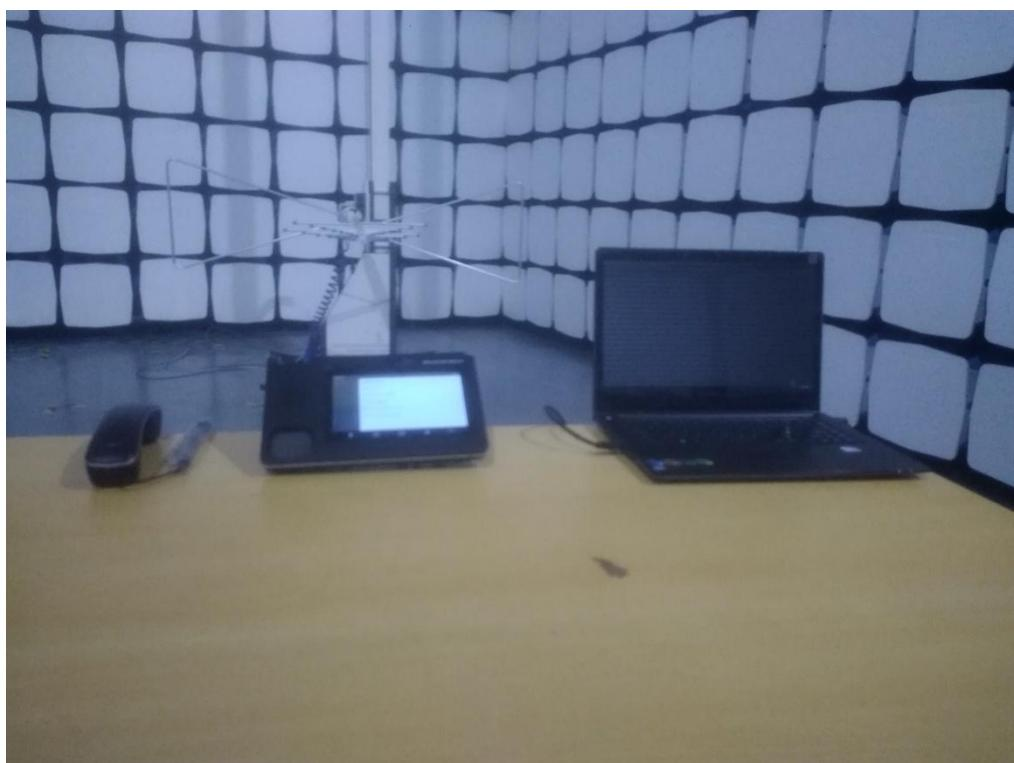
**Radiated Emission test view (Frequency above 1GHz)**
