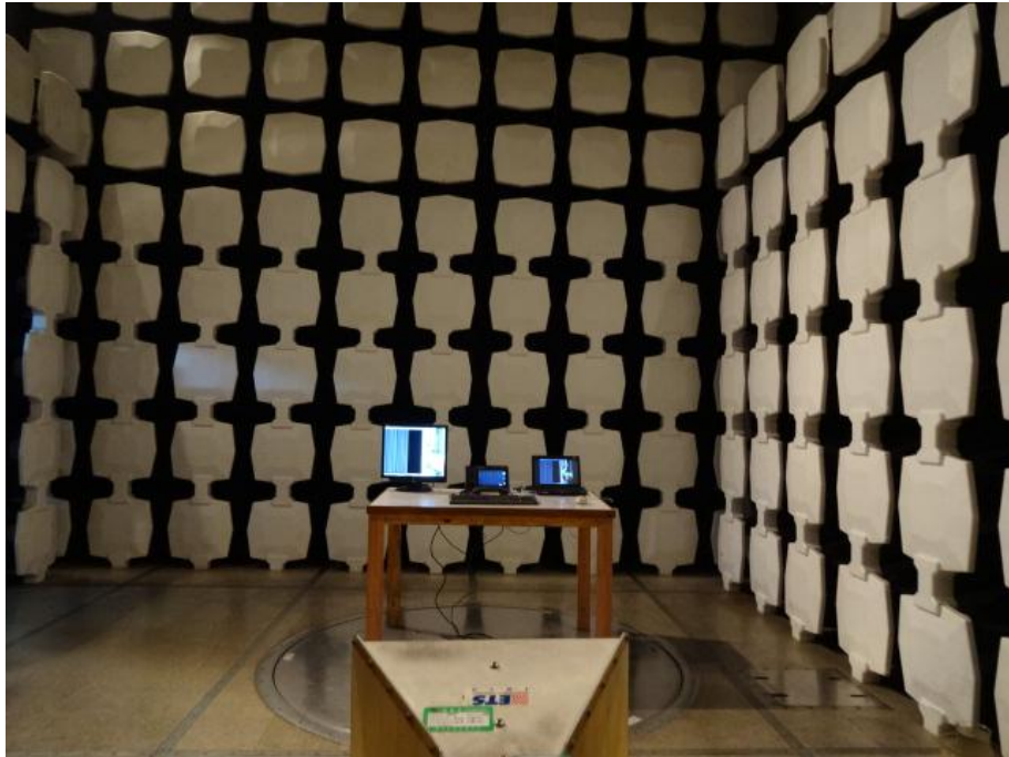
Radiated Emission Test Set-up (Above 1GHz)
