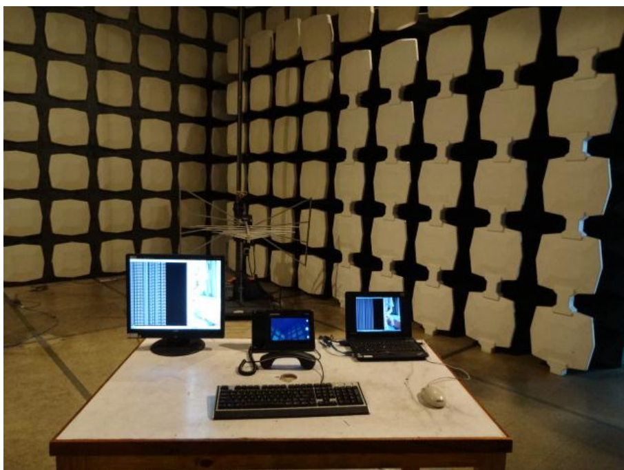
Radiated Emission Test Set-up (Below 1GHz)
