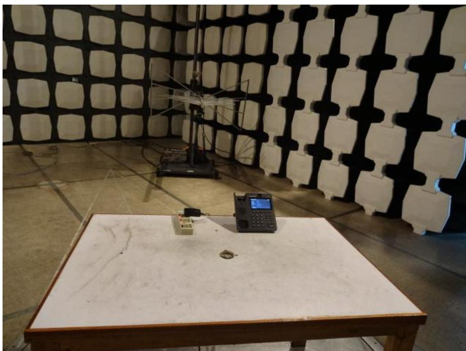
**Radiated Emission Test Set-up - beLowest 1GHz**
