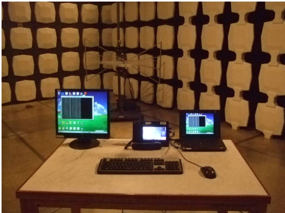
Radiated Emission Test Set-up (Below 1GHz)
