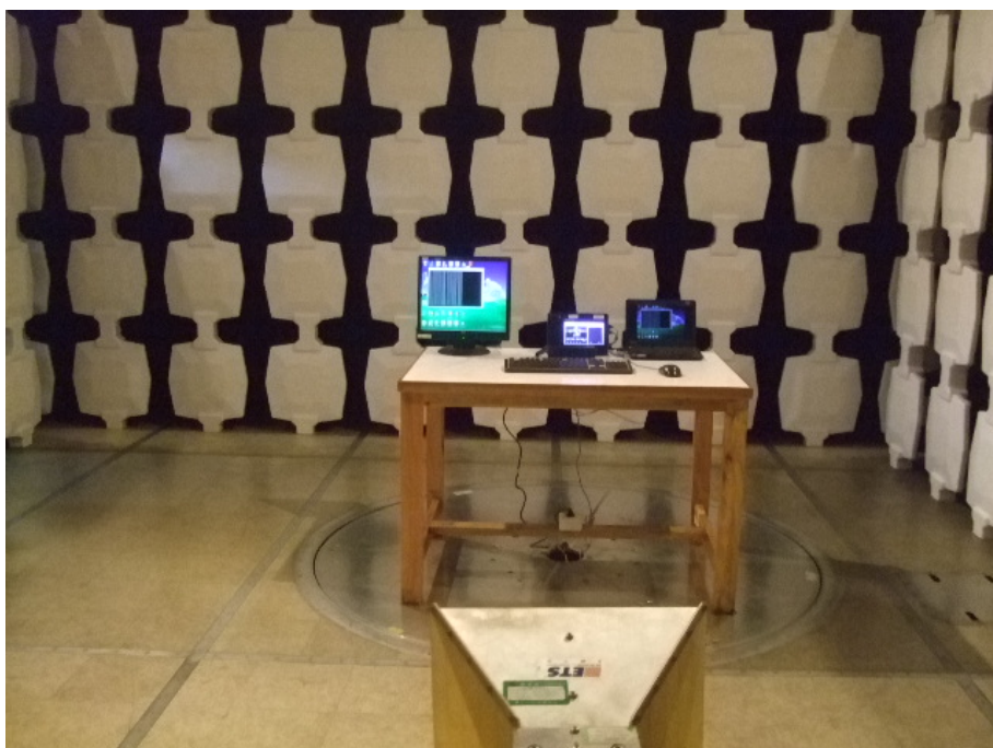
Radiated Emission Test Set-up (Above 1GHz)
